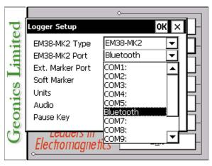
When Bluetooth connection is selected and Logger Setup is closed with OK button and other survey parameters are specified, please proceed and tap (or execute by keyboard) option Monitor/Log. <u>At that time the EM38-MK2 must be **ON**</u>.
