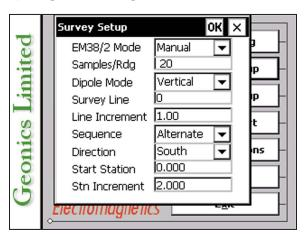
This parameter describes number of readings that will be taken after the trigger switch is pressed. At the end of sampling time the logger will beep and an average value will be written in to the file and plotted on the screen. During the sampling period interval data are measured at approximately 20 readings per second. For example by specifying 10 samples, 0.5 second will be used at each station. The maximal sampling is 100 readings which corresponds to approximately 5 seconds at each station.
