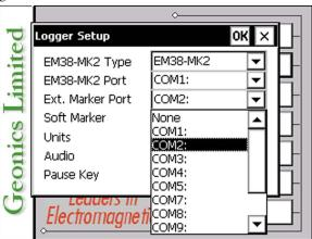
This port must be different than the port specified in the Set Port for GPS option (see next chapter), otherwise a message will be displayed and the ports will have to be reassigned. If External Marker is located on the Extender Arm then The EM38-MK2 and Ext. Marker Port must be the same (usually COM1 or COM2).
