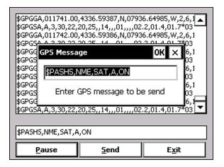
After this command is received by the GPS receiver, the confirmation message will be send by the receiver (\$PASHR, ACK\*3D) and data stream will contain the message SAT (\$PASHR, SAT,..... in the above figure).
