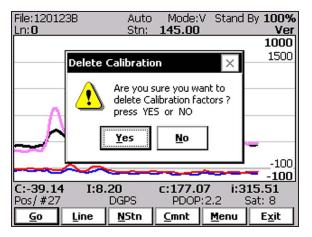
Please confirm by tapping button **Yes**, or pressing Key **Y** or Enter (if button **Yes** is highlighted) to delete (reset) calibration factors. After this is done readings displayed by the instrument console and Allegro should be similar.
