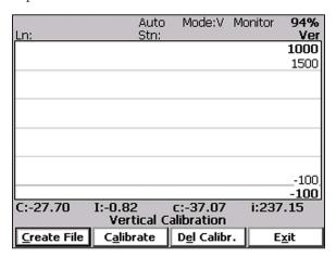
After Vertical calibration is completed (usually few seconds) the program will beep and a message **Rotate to Horizontal mode within 60 seconds** will appear.
