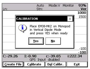
After the instrument is placed on the monopod in Vertical dipole mode tap button **Yes** or press key **Y** (or **Enter** if button is highlighted). After button **Yes** was tapped a messages box disapears and a prompt **Vertical Calibration** is displayed. From now on all mesages and prompts will be written under plot section of the screen, in a line that is normally used to display GPS parameters.
