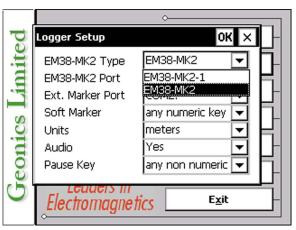
between the models is the number of included receiver coils: the EM38-MK2-1 includes one receiver coil with a 1 meter transmitter / receiver intercoil spacing; the EM38-MK2 includes two receiver coils with 0.5 and 1 meter intercoil spacings. The program default is the EM38-MK2.
