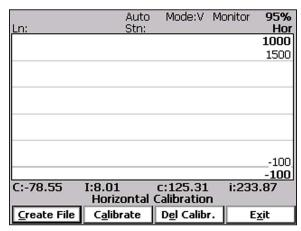
If for any reason the calibration is not successfull a proper message will be displayed. Horizontal calibration takes normally 2 seconds and when the procedure is completed a confirmation message will be displayed.
