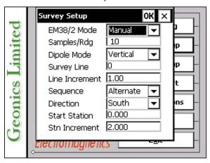
In Manual Mode any combination of dipole modes (Vertical, Horizontal or Both) can be selected.
