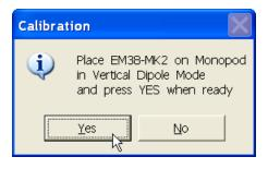
After the instrument is placed on the monopod in Vertical dipole mode click on the button **Yes** or press key **Y** (or **Enter** if button is highlighted). After button **Yes** was clicked a messages box disapears and a prompt **Vertical Calibration** is displayed. From now on all messages and prompts will be written under plot section of the screen, in a line that is normally used to display labels for EM38-MK2 readings.
