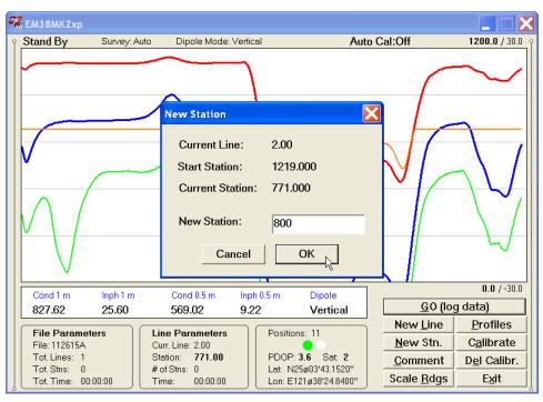
updated and after data logging is activated the profile curves will have a small gap (two pixels) showing the new station entry (see Figure below).
