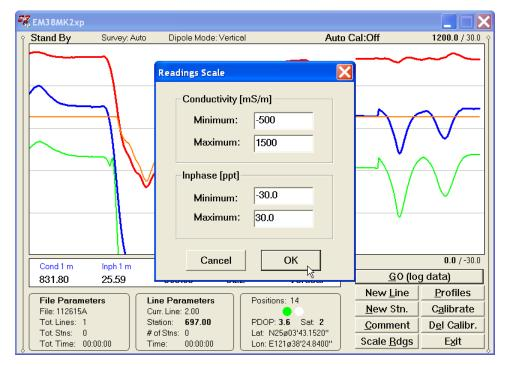
Current settings (minimum and maximum values) for the scale are displayed in the bottom right and top right corners of the plot area (Conductivity/Inphase). Values displayed in bold indicate the scale that is associated with grey grid lines.
