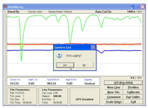
After the above message is confirmed the program stops logging, closes the data file and returns to the Main Screen.
