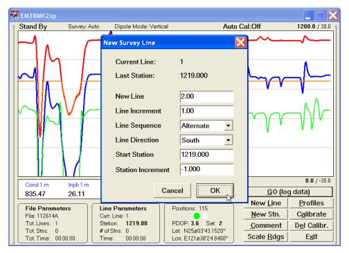
At the top of the dialog the last survey line name and the last logged station are displayed. Default name for the new line is given based on the Line Increment parameter. The default Start Station, direction of the Station Increment, and Direction are determined based on Sequence selection. All these parameters can be overwritten by the user as described in the Survey Setup menu description (chapter 2).
