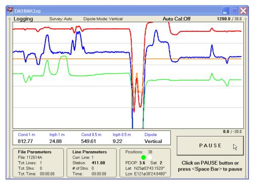
After the screen changes to Logging mode the current station (label **Stn:**) is updated according to the station interval. Similarly, if GPS Input was enabled, total number of GPS positions (label **Positions**) in the data file is incremented every time (usually once a second) GPS position is written to the file. Profile curves (for channels selected in Display Options window) are updated after each reading is written to the data file.
