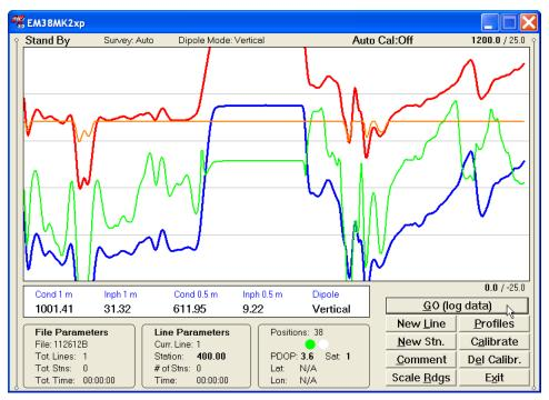
Parameters frame contains: name of current survey line, current station, number of stations in the current survey line, and time of surveying current line. In the Stand By mode the station number will not change. Stations in the EM38-MK2 program are incremented by station increment value after each reading is written to the data file.
