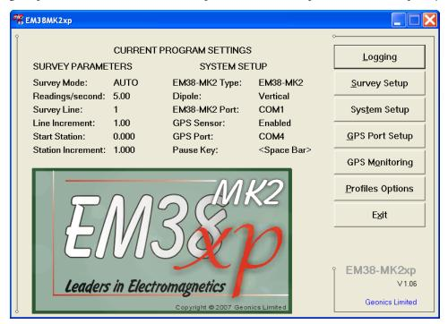
and a data file can be created. The instrument can be also calibrated in Monitoring mode. After a data file is created in Monitoring mode, the program switches to Stand By mode and allows access to Logging mode. In Stand By mode instrument output can be monitored and some survey and logging parameters can be changed, and the Logging mode is used only to record data. Two modes Stand By and Logging are toggled by **GO** and **Pause** buttons.
