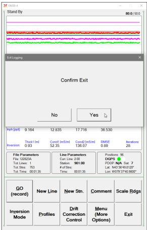
After above message is confirmed the program stops logging, closes data file and returns to Main Screen.
