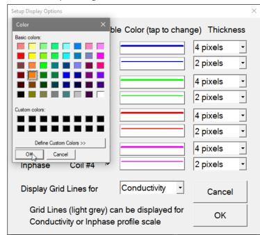
Click on the button **OK** or press **ENTER** key to accept the highlighted colour. The Color dialog will disappear and the colour of the appropriate channel button will updated. To cancel colour selection click **Cancel** (X) button or press **Esc** key.
