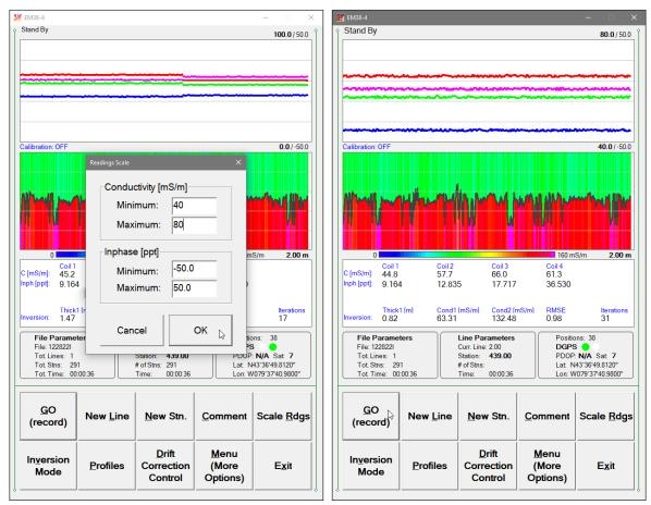
and Inphase. Current settings (minimum and maximum values) for the scale are displayed in the bottom right and top right corners of the plot area (Conductivity/Inphase). Values displayed in bold indicate the scale that is associated with grey grid lines. After minimum and maximum values are specified click on the button **OK** or press **ENTER** key to accept new values and the profile plot area will be redrawn (see Figure above on the right).
