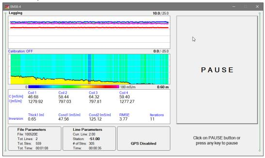
After all the parameters in the System Setup dialog are updated click on the button **OK** or press **ENTER** key to accept the displayed settings. The program will return to the Main Screen. Updated settings will be written to the initial file and they will be given as default parameters in the subsequent System Setup dialog.
