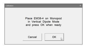
After the instrument is placed on the monopod in Vertical dipole mode click on the button **Yes** or press key **Y** (or **Enter** if button is highlighted). After button **Yes** was clicked a messages box disappears and a prompt **Vertical Calibration** is displayed (Figure below, on the left). From now on all messages and prompts will be written under plot section of the screen, in a line that is normally used to display labels for EM38-4 readings.
