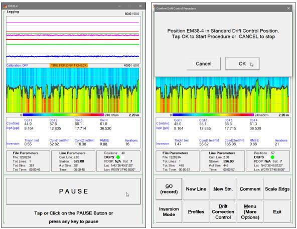
After the Drift Correction Control button is tapped a dialog labeled Confirm Drift Control Procedure appears (see above, the Figure on the right). In case the button was tapped or pressed accidentally then just tap on the Cancel button and the EM38-4 program will return to Stand By mode operation. Otherwise, position the instrument as described above and tap the OK button to start the Drift Control procedure.
