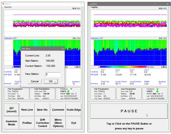
To return to Stand By mode and current survey line settings (state before this dialog was selected) click on the **Cancel** (X) button or press **Esc** key, the dialog window will disappear and measurements can be continued.
