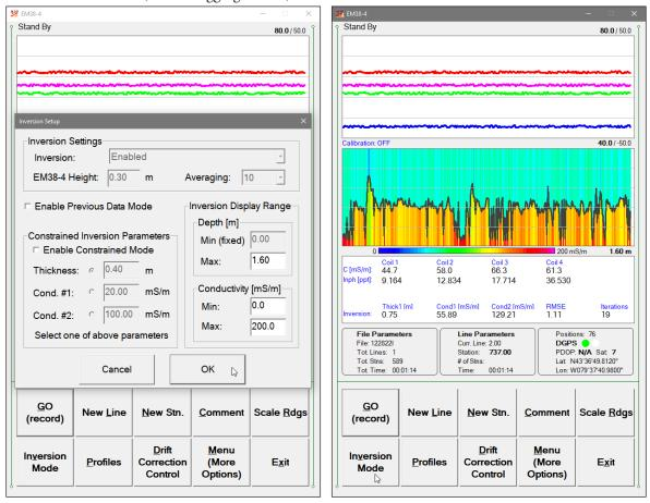
The option Enable Previous Data Mode is now enabled, it was disabled while the dialog was displayed in the Main Screen mode. When enabled this option uses current as well as previous data during inversion calculations. Example with modified scale for Inversion conductivity results is displayed in Figure above, on the right.
