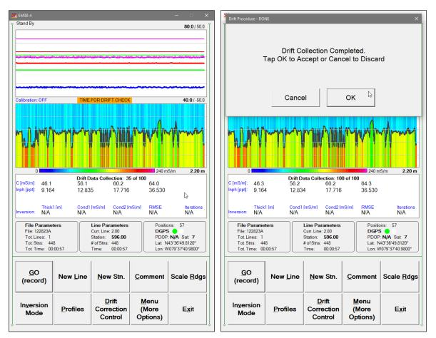
the data file. Parameters recorded during the Drift Correction Control procedure can be used later while processing data file in the DAT38-4 program.
