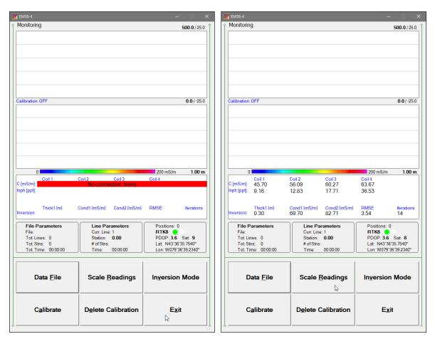
Check the connection or turn the instrument ON and the "No Connection" message will disappear and measured values will be displayed (Figure above on the right).
