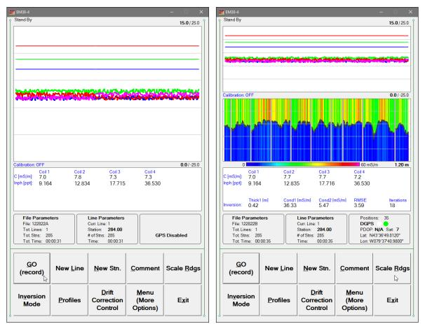
A section of the window at the top of the screen contains one line of text displaying survey and instrument related parameters. These are: logging mode (**Stand By** or **Logging**) and when fiducial marker is active a label **Marker** is displayed in this line. Auto Calibration state is indicated by a label located below profile graph window **Calibration: ON** (performed and active) or **Calibration: OFF** (not used).
