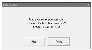
Please confirm by tapping button **Yes**, or pressing Key **Y** or Enter (if button **Yes** is highlighted) to delete (reset) calibration factors. After this is done readings displayed by the instrument console and the logging computer should be similar.
