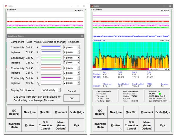
Please refer to chapter 5 where this dialog and its parameters are described in detail. Click on the button **OK** or press **ENTER** key to accept updated display parameters. The dialog will disappear and profile plot area will be redrawn in Stand By mode.
