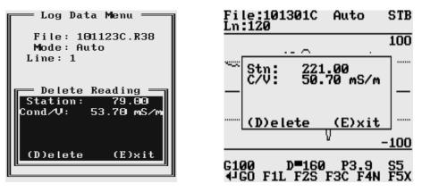
This function allows operator to delete previously recorded reading(s). The reading (station) to be deleted is displayed on the screen. The data will only be deleted when the key  $\mathbf{D}$  is pressed. The program will then display the next previous station, and allow it to be deleted in a similar fashion. If there is no further data available, the program will provide related information.
