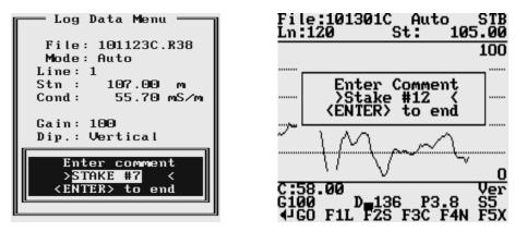
Selecting this option allows the operator to enter a comment at any point of the survey. A maximum of 11 characters can be entered as a comment. Text of the comment is saved in the file with a corresponding time stamp.
