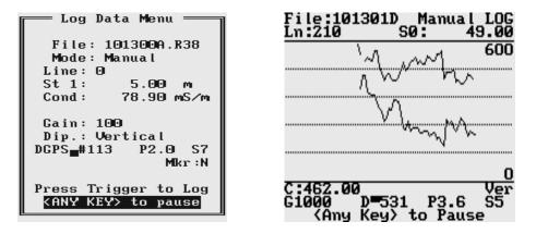
There is only one option available in the Logging mode - pause logging. After a Pause key (any key, Alt+F1, or Ctrl+F5) selected in Logger Setup menu is pressed the recording is stopped and the Log Data menu returns to the Stand By mode. The EM38 data will be displayed with the update rate approximately 10 readings per second, however data will not be saved in the log file, audible click will stop if Sound option was enabled, and if graphic mode is used, profile curves will not be updated.
