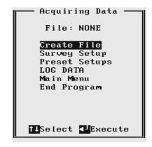
At the top of the screen the current name of the data file is displayed. If data file is not created its name is displayed as NONE. The menu contains several options listed below.
