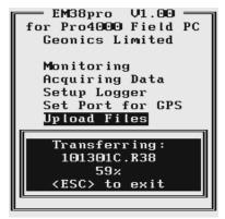
Transferred files (in EM38pro format) will be displayed in the centre list box. After the transfer of all selected files is complete, files in the EM38pro format are automatically converted to the DAT38 format (with extension name G38). Converted files will be displayed in the Converted Files list box (see Figure below). Converted files (with extension name G38) can be loaded and processed further in the program.
