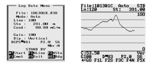
The main portion of the screen in graphic mode is occupied by the plot area. Readings in the plot area can be displayed in the user specified scale. The amplitude scale is divided by four or five dotted grid lines. In cases where the amplitude scale starts with a negative value, then the grid line corresponding to zero is always plotted as a solid line.
