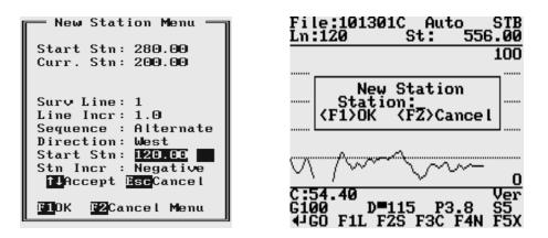
Pressing key F2 or <Esc> will disregard new entry and the program will return to the Log Data screen and measurements can be continued.
