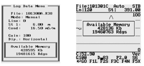
Available memory is also checked automatically during data collection. In cases where the amount of available memory in the logger is less than 10 Kbytes, the program will stop, data file will close, and a proper message will be displayed.
