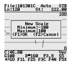
Selecting this option allows the operator to enter new scale parameters for the amplitude display. After minimum and maximum values are specified, the function key **F1** (OK) will accept new values and the display will be redrawn (see below). When the key **F2** (Cancel) is pressed the new entry is cancelled.
