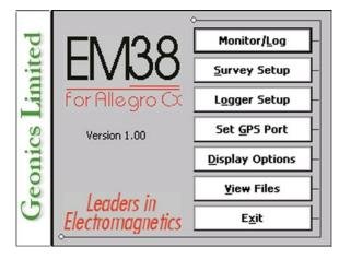
and GPS parameters can be quickly examined and creating data file can be performed. After a data file is created in Monitoring mode, the program switches to Stand By mode and allows access to Logging mode. In Stand By mode instrument output can be monitored and some survey and logging parameters can be changed, and Logging mode is used only to record data. Two modes Stand By and Logging are toggled by **GO** and **Pause** buttons.
