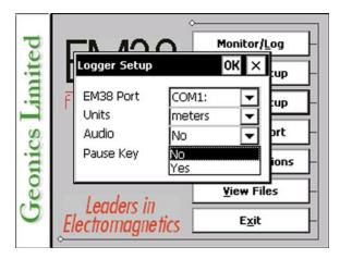
pause data recording during logging session. Default setting **any key** can be changed to one of the three specific keys for field conditions where a logger key can be accidentally pushed causing unwanted stop of data logging.
