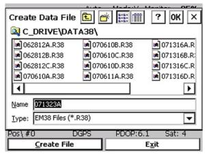
The file name can be specified in the Create Data File dialog using the Windows standard interface procedure. The EM38 data files cannot be appended.
