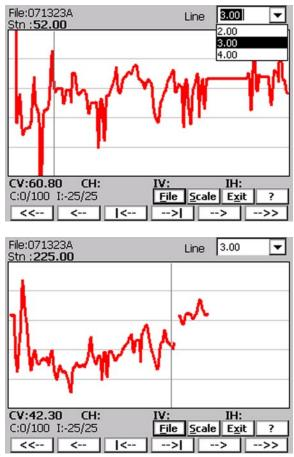
To shift the range of the displayed stations and to move the vertical bar indicating the currently displayed station, use the buttons located along the bottom of the View Files window. These buttons can be activated by tapping or by pressing the keyboard keys. A help screen containing info related to each button can be displayed at any time by tapping (or executing from keyboard) the Help button labeled ?. The Help screen is shown below.
