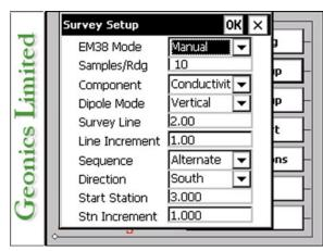
This parameter describes number of readings that will be taken after the trigger switch is pressed. At the end of sampling time the logger will beep and an average value will be written in to the file and plotted on the screen. During the sampling period interval data are measured at approximately 10 readings per second. For example by specifying 10 samples, 1 second will be used at each station. The maximal sampling is 100 readings which corresponds to approximately 10 seconds at each station.
