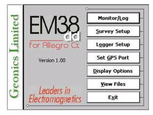
gain, and GPS parameters can be quickly examined and creating data file can be performed. After a data file is created in Monitoring mode, the program switches to Stand By mode and allows access to Logging mode. In Stand By mode instrument output can be monitored and some survey and logging parameters can be changed, and Logging mode is used only to record data. Two modes Stand By and Logging are toggled by **GO** and **Pause** buttons.
