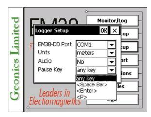
After all the parameters in the Logger Setup dialog are updated tap the button **OK** or press **ENTER** key to accept the displayed settings. The program will return to the Main Screen. Updated settings will be written to the initial file and they will be given as default parameters in the subsequent Logger Setup dialog.
