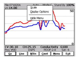
Options listed in the menu can be accessed directly (without displaying pop up menu from Menu button) by using keyboard shortcuts, i.e. pressing key **S** will display Scale dialog. While menu is displayed options can be selected by tapping on the appropriate proper option, or from the keyboard by pressing the shortcut keys or by navigating using  $\langle Up \rangle$  and  $\langle Down \rangle$  arrow keys and executing by  $\langle ENTER \rangle$
