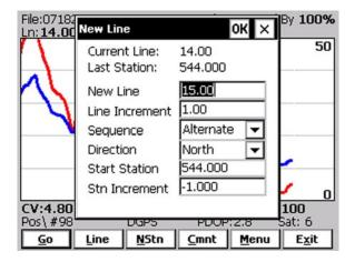
At the top of the dialog the last survey line name and the last logged station are displayed. Default name for the new line is given based on the Line Increment parameter. The default Start Station, direction of the Station Increment, and Direction are determined based on Sequence selection. All these parameters can be overwritten by the user as described in the Survey Setup menu description (chapter 2).
