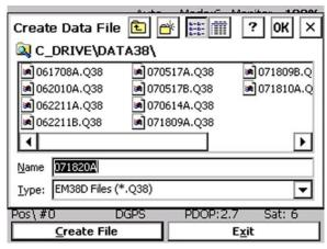
The file name can be specified in the Create Data File dialog using the Windows standard interface procedure. The EM38DD data files cannot be appended.
