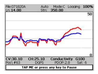
After the screen changes to Logging mode the current station (label **Stn:**) is updated according to the station interval. Similarly, if GPS Input was enabled, total number of GPS positions (label **Pos**) in the data file is incremented every time (usually once a second) GPS position is written to the file. Profile curves (for channels selected in Display Options window) are updated after each reading is written to the data file.
