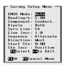
To select any option use the **Down** and **Up** keys. To start the editing of any setting press **Left** or **Right** key. Some parameters that have only a few possible options (e.g. EM38 Mode) can be simply toggled by **Left** or **Right** keys.
