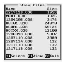
Select the file by using **Down** and **Up** arrow keys. When the desired file is highlighted press function key **F1** to view contents of this file. Pressing key **F2** will return the program to the EM38Dpro Main menu.
