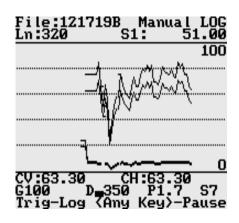
There is only one option available in the Logging mode - pause logging. After a Pause key (any key, Alt+F1, or Ctrl+F5) selected in Logger Setup menu is pressed the recording is stopped and the Log Data menu returns to the Stand By mode. The EM38DD data will be displayed with the update rate approximately 10 readings per second, however data will not be saved in the log file, audible click will stop if Sound option was enabled, and if graphic mode is used, profile curves will not be updated.
