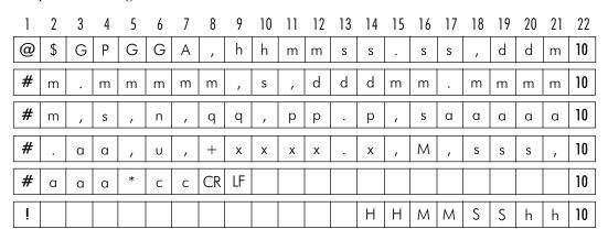
The GPS sequence may contain 5 or 6 records. Component of the GGA message may differ in length, however they are placed in the same number of columns. Refer to Appendix A (section A.2) for definition of each component of GGA data message.
