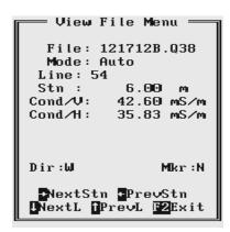
At the top of the screen name of the data file and the EM38DD mode are displayed. Then the Line Name, Station, and readings with the instrument component (conductivity or Inphase) are shown. The survey line direction (Dir) and the fiducial marker (Mkr) presence  $\mathbf{Y}(es)$  or  $\mathbf{N}(o)$  are displayed as well. If the file contains comments, the text will be displayed between neighbouring stations.
