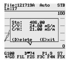
This function allows operator to delete previously recorded reading(s). The reading (station) to be deleted is displayed on the screen. The data will only be deleted when the key  $\mathbf{D}$  is pressed. The program will then display the next previous station, and allow it to be deleted in a similar fashion. If there is no further data available, the program will provide related information.
