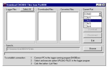
To start downloading the data files, connect the field computer (Pro4000) and PC computer with the serial cable.
