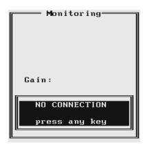
Check the connection or turn the instrument ON and select the Monitoring option again.
