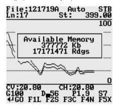
Available memory is also checked automatically during data collection. In cases where the amount of available memory in the logger is less than 10 Kbytes, the program will stop, data file will close, and a proper message will be displayed.
