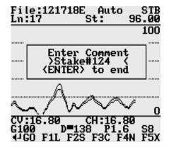
Selecting this option allows the operator to enter a comment at any point of the survey. A maximum of 11 characters can be entered as a comment. Text of the comment is saved in the file with a corresponding time stamp.
