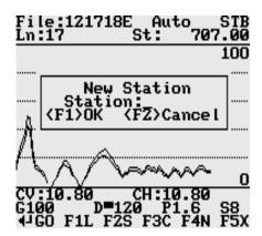
Pressing key F2 or <Esc> will disregard new entry and the program will return to the Log Data screen and measurements can be continued.
