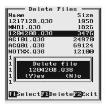
If key **Y** will be pressed the file will be permanently deleted from the field computer memory. When key **N** is pressed the confirmation prompt disappears and display shows the list of available data files.
