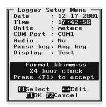
The modified time is accepted (and set in the computer clock) after the function key **F1** is pressed.
