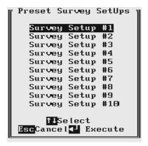
To select any survey set up number use **Down** and **Up** keys, and to start editing particular Survey Setup menu press **ENTER**>. Press **Esc**> key. to return to the Acquiring Data menu.
