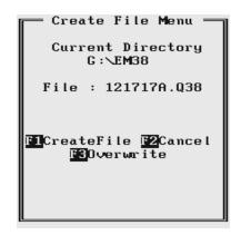
The file can be created by pressing the function key **F1**, this option can be skipped by pressing the function key **F2**., or by pressing key **F3** the file name can be overwritten. After key **F3** is pressed the Create File menu will be displayed as follows.
