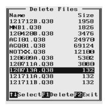
Select the file by using **Down** and **Up** arrow keys. When the file to be deleted is highlighted press function key **F1** to delete the file. Pressing key **F2** will return the program to the EM38Dpro Main Menu.
