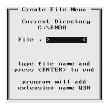
Each data file in the field computer (raw data file) has an extension name Q38 and it is created in the programs current directory. The Q38 files are created in the instrument binary format. They can be viewed using the Main menu option "View Files". These files can be also converted to ASCII format and processed in the Geonics program DAT38DDW and DAT38DM (for DOS).
