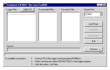
The Download window has three list boxes. The first from the left, labeled Logger Files will contain, after the **List Files** button is clicked, a list of data files located in the field computer and available
