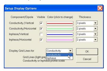
Minimum and maximum values for the component with selected grid lines are displayed as bold numerals. See figure below where grid lines are plotted for conductivity scale.
