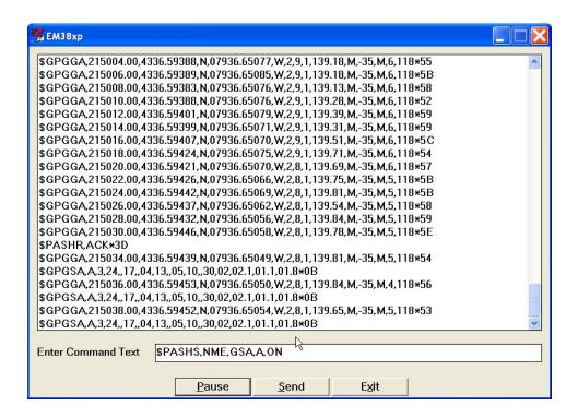
Please note, that not every GPS system accepts and uses the same standard set of NMEA commands and messages. In addition, some GPS systems do not accept commands sent by the serial port at all. The configuration of these type of receivers can be updated only by the controlling device (usually GPS logger, controller, or the receiver panel keys).
