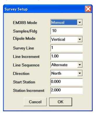
This parameter describes number of readings that will be taken after the trigger switch is pressed. At the end of sampling time the logger will beep and an average value will be written in to the file and plotted on the screen. During the sampling period interval data are measured at approximately 10 readings per second. For example by specifying 10 samples, 1 second will be used at each station. The maximal sampling is 100 readings which corresponds to approximately 10 seconds at each station.
