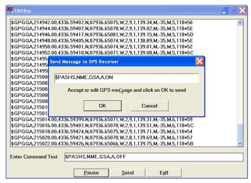
After this command is received by the GPS receiver, the confirmation message will be send by the receiver (\$PASHR, ACK\*3D) and data stream will contain the message GSA (\$PASHR, NME,GSA,A,ON), see Figure below.
