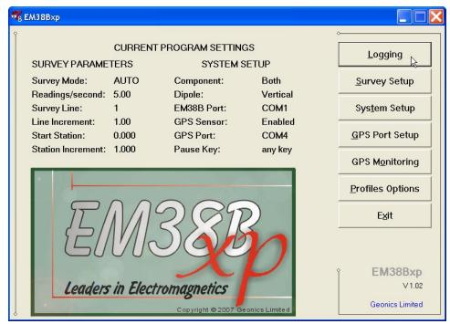
After a data file is created in Monitoring mode, the program switches to Stand By mode and allows access to Logging mode. In Stand By mode instrument output can be monitored and some survey and logging parameters can be changed, and Logging mode is used only to record data. Two modes Stand By and Logging are toggled by **GO** and **Pause** buttons.
