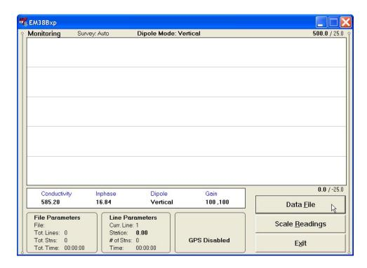
The remaining bottom section contains a window with current EM38B readings (Conductivity and Inphase, dipole mode, and Gain), three frames (File Parameters, Line Parameters, and GPS information), and command buttons located on the right side of the screen.
