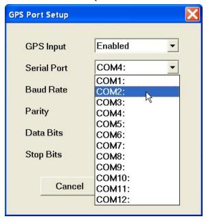
This port must be different than the port specified in the System Setup menu (for EM38B), otherwise a message will be displayed and ports will have to be reassigned.
