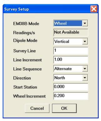
Please note that while in former data acquisition system (DAS70) Stn Increment (station increment) had only two options: Positive or Negative, in the current program this parameter is optional and its value has to be entered according to used wheel increment.
