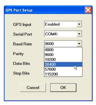
Clicking on the down arrow next to the text box labeled Baud Rate opens a drop-down box showing the available parameters, or when the keyboard is used activate this text box by pressing TAB key and then by using up or down arrow keys select one of available items.
