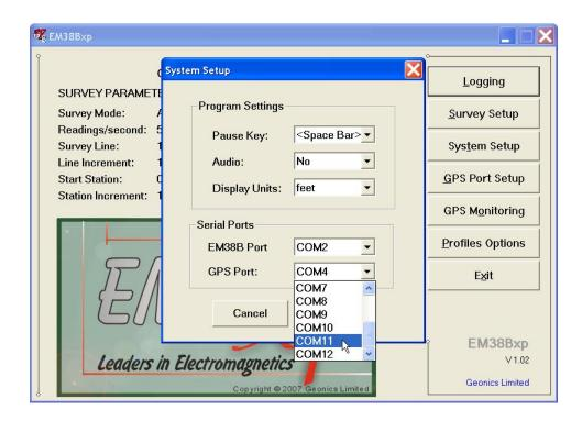
After all the parameters in the System Setup dialog are updated click on the button **OK** or press **ENTER** key to accept the displayed settings. The program will return to the Main Screen. Updated settings will be written to the initial file and they will be given as default parameters in the subsequent System Setup dialog.
