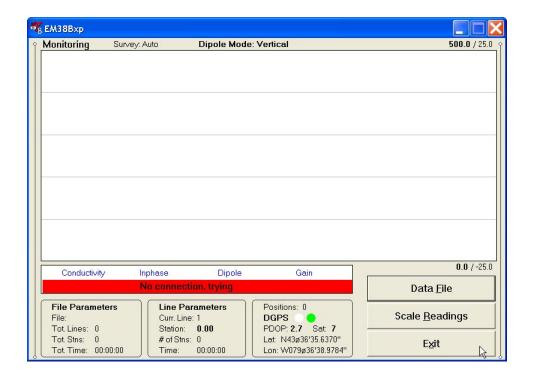
tor, Stand By or Logging), survey mode (Auto, Wheel, or Manual), and user specified instrument dipole mode (Vertical, Horizontal or Both following label **Dipole Mode:**). When fiducial marker is pressed then **M** is displayed.
