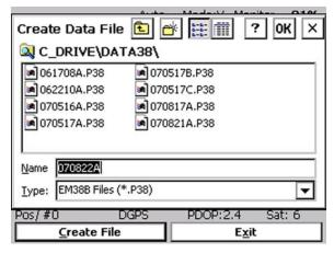
The file name can be specified in the Create Data File dialog using the Windows standard interface procedure. The EM38B data files cannot be appended.
