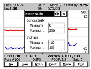
After minimum and maximum values are specified tap the button **OK** or press **ENTER** key to accept new values and the profile plot area will be redrawn (see Figure below).
