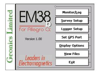
These options are selected by using tapping buttons, or from keyboard using TAB/ENTER or shortcuts indicated by underline label characters. In case of Main Screen buttons the **Down** and **Up** arrow keys and **<ENTER**> can be used as well.
