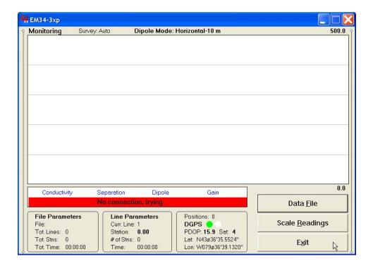
tor, Stand By or Logging), survey mode (Auto, Wheel, or Manual), and user specified instrument dipole mode and coil separation (following label **Dipole Mode:**). When fiducial marker is pressed then **M** is displayed.
