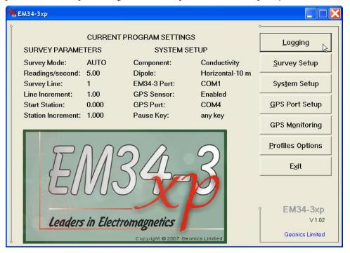
can be created. After a data file is created in Monitoring mode, the program switches to Stand By mode and allows access to Logging mode. In Stand By mode instrument output can be monitored and some survey and logging parameters can be changed, and Logging mode is used only to record data. Two modes Stand By and Logging are toggled by **GO** and **Pause** buttons.
