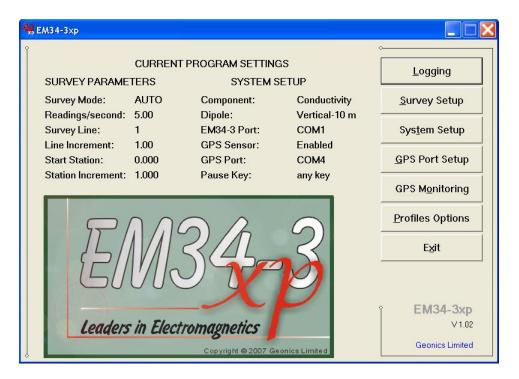
The Main Screen appears always as the first window after the program is started. It contains the name of the program, its version number (right bottom corner), and list of command buttons with available options on the right side. The major, left portion of the window contains information about current survey and system settings. This section is updated in real time as soon as the program parameters are changed in dialogs.
