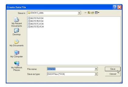
The file name can be specified in the Create Data File dialog using the Windows standard interface procedure. The EM34-3 data files cannot be appended.
