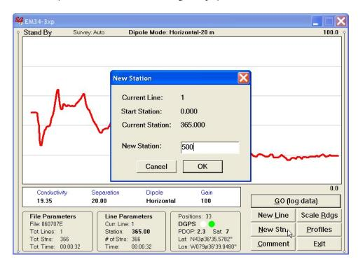
Current survey line, Start and Current station are displayed at the top of the dialog. The New Station can be entered in the provided edit box labeled New Station.
