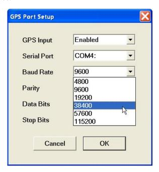
Clicking on the down arrow next to the text box labeled Baud Rate opens a drop-down box showing the available parameters, or when the keyboard is used activate this text box by pressing TAB key and then by using up or down arrow keys select one of available items.
