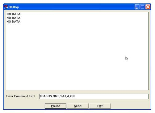
The message NO DATA is normally updated with a rate of 7 seconds. This may indicate the following: serial port number not correctly specified in Set Port for GPS dialog, GPS receiver not sending any data, and not working or not connected GPS receiver. If the message is updated more often than 7
