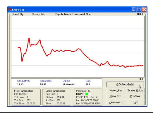
The main portion of the screen is occupied by the plot area which displays profiles (see Figure below which shows Stand By mode after some data were collected). Scale for conductivity is labeled at the top and bottom of the plot window. The amplitude scale is divided by three to five grey grid lines. In the case where the amplitude scale starts with a negative value, then the grid line corresponding to zero is always plotted as a thicker line.
