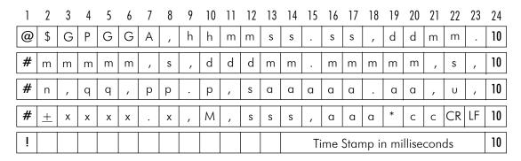
The GPS sequence may contain 4 to 6 records. Component of the GGA message may differ in length, however they are placed in the same number of columns. Refer to Appendix B (section B.2) for definition of each component of GGA data message.
