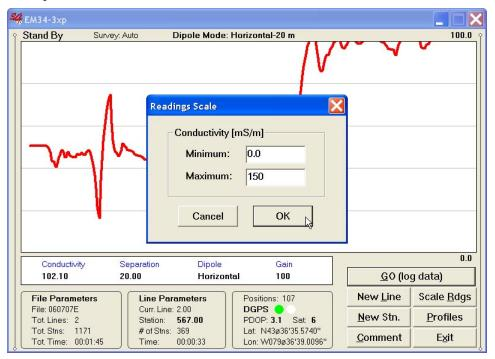
After minimum and maximum values are specified click on the button **OK** or press **ENTER** key to accept new values and the profile plot area will be redrawn (see Figure below).
