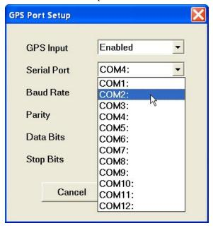
This port must be different than the port specified in the System Setup menu (for EM34-3), otherwise a message will be displayed and ports will have to be reassigned.
