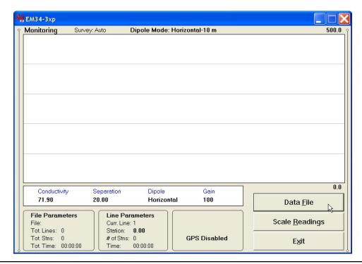
The EM34-3 readings and other parameters are displayed from the left in order: Conductivity reading in mS/m, and associated current coil separation, current dipole mode, and the EM34-3 range (labeled Gain). The EM34-3 readings are updated approximately 10 times per second during the monitoring session.
