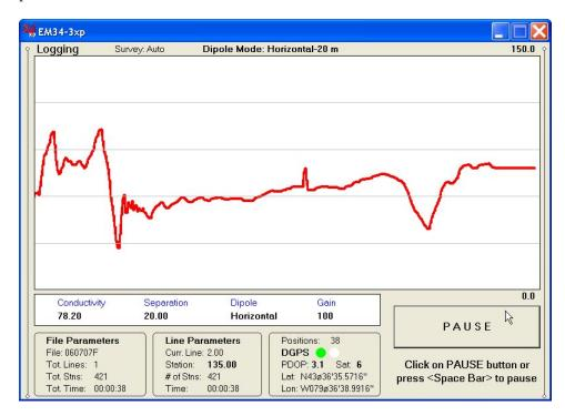
After the screen changes to Logging mode the current station (label **Stn:**) is updated according to the station interval. Similarly, if GPS Input was enabled, total number of GPS positions (label **Positions**) in the data file is incremented every time (usually once a second) GPS position is written
