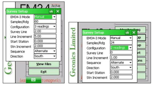
This parameter describes number of readings that will be taken after the trigger switch is pressed. At the end of sampling time the logger will beep and an average value will be written in to the file and plotted on the screen. During the sampling period interval data are measured at approximately 10 readings per second. For example by specifying 10 samples, 1 second will be used at each station. The maximal sampling is 100 readings which corresponds to approximately 10 seconds at each station.
