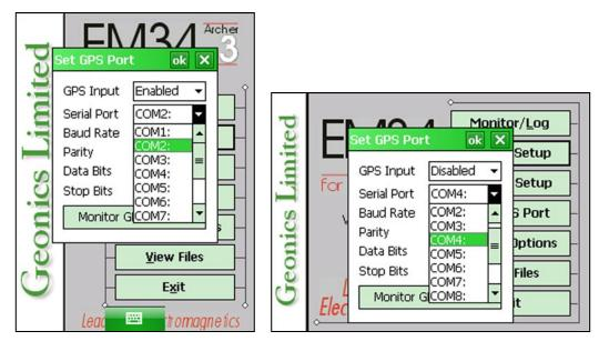
If Bluetooth communication is employed between Archer and GPS receiver please use serial port that has been assigned by Windows Mobile operating system to the Bluetooth connection.
