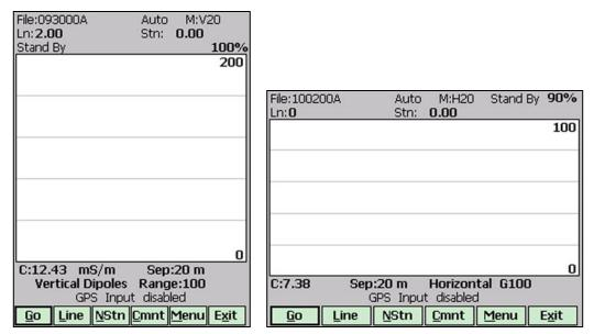
The main portion of the screen is occupied by the plot area which displays profiles (see Figure below which shows Stand By mode after some data were collected). Scale for conductivity is labeled at the top and bottom (on the right) of the plot window. The amplitude scale is divided by three to five grey grid lines. In the case where the amplitude scale starts with a negative value, then the grid line corresponding to zero is always plotted as a thicker line.
