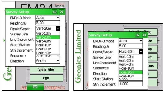
If Manual mode was selected six settings are available as well: 1, 2, 3, 4, 5, or 6. In this case the selected number describes number of different instrument configurations to be taken at each station. Readings at each station can be taken in any order, however care should be taken to collect desired type and number of configurations at each station.
