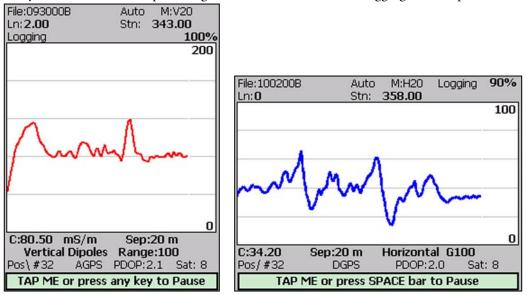
After the screen changes to Logging mode the current station (label **Stn:**) is updated according to the station interval. Similarly, if GPS Input was enabled, total number of GPS positions (label
