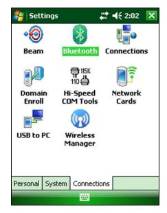
After tapping on the Bluetooth icon the following screen will appear. Tap on the Add new device item. <u>At that time the EM38-MK2 must be **ON**</u>.
