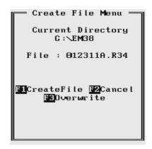
The file can be created by pressing the function key **F1**, this option can be skipped by pressing the function key **F2**., or by pressing key **F3** the file name can be overwritten. After key **F3** is pressed the Create File menu will be displayed as follows.
