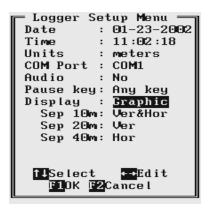
Parameter **Sep 10m** (coil separation 10 m), and similarly **Sep 20m** and **Sep 40m**, allow you to enable display of Vertical (**Ver**), Horizontal (**Hor**), both (**Ver&Hor**), or **None** dipole modes separately.
