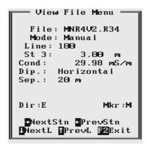
At the top of the screen name of the data file and the EM34 mode are displayed. Then the Line Name, Station, and readings with the instrument dipole mode (V for Vertical or H for Horizontal) and coil separation (10, 20, or 40 m) are shown. The survey line direction (Dir) and the fiducial marker (Mkr) presence  $\mathbf{Y}(es)$  or  $\mathbf{N}(o)$  are displayed as well. If the file contains comments, the text will be displayed between neighbouring stations.
