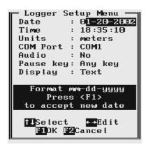
The new date is accepted (and set in the computer) after the function key **F1** is pressed. Use **Down** or **Up** arrow key to exit the editor and cancel any changes.
