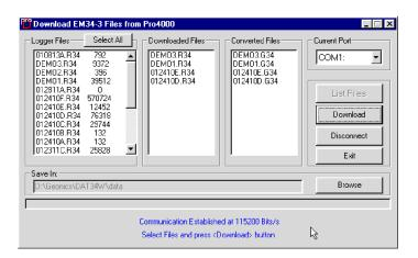
Click the **Disconnect** button to cancel communication with logger. The Download EM34-3 Files from Pro4000 window will remain on the screen and next data transfer session (i.e. from another logger) can be performed. Clicking the **Exit** button will stop Data Transfer function and the Download EM34-3 Files from Pro4000 window will disappear.
