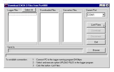
The Download window has three list boxes. The first from the left, labeled Logger Files will contain, after the **List Files** button is clicked, a list of data files located in the field computer and available to download. File names, with their size in bytes will be displayed as well. The second list box,
