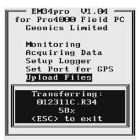
Transferred files (in EM34pro format) will be displayed in the centre list box. After the transfer of all selected files is complete, files in the EM34pro format are automatically converted to the DAT34 format (with extension name G34). Converted files will be displayed in the Converted Files list box (see Figure below). Converted files (with extension name G34) can be loaded and processed further in the program.
