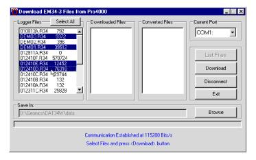
When file selection is complete click the **Download** button. The name of each transferred file is displayed at the bottom of the window as it transfers and a progress bar indicates the percentage completed, as shown in the following Figure.
