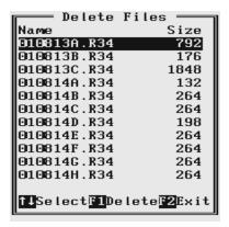
Select the file by using **Down** and **Up** arrow keys. When the file to be deleted is highlighted press function key **F1** to delete the file. Pressing key **F2** will return the program to the EM31pro Main Menu.
