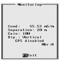
The EM34-3 readings are updated approximately 10 times per second during monitoring session. Values of conductivity in mS/m are displayed. The dipole mode, coil separation, instrument scale, and state of fiducial marker are continuously updated.
