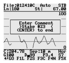
Selecting this option allows the operator to enter a comment at any point of the survey. A maximum of 11 characters can be entered as a comment. Text of the comment is saved in the file with a corresponding time stamp.
