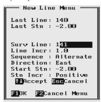
At the top of the screen the last survey line name and the last station are displayed. Default name for the new line is given based on the Line Increment parameter. The default Start Station, direction of the Station Increment, and Direction are determined based on Sequence selection. All these parameters can be overwritten by the user as described in the Survey Setup menu description (section 9.2).
