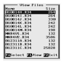
Select the file by using **Down** and **Up** arrow keys. When the desired file is highlighted press function key **F1** to view contents of this file. Pressing key **F2** will return the program to the EM34pro Main menu.
