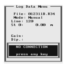
Check the connection or turn the instrument ON and select the LOG DATA option again.
