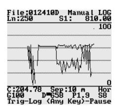
There is only one option available in the Logging mode - pause logging. After a Pause key (any key, Alt+F1, or Ctrl+F5) selected in Logger Setup menu is pressed the recording is stopped and the Log Data menu returns to the Stand By mode. The EM4-3 data will be displayed with the update rate approximately 10 readings per second, however data will not be saved in the log file, audible click will stop if Sound option was enabled, and if graphic mode is used, profile curves will not be updated.
