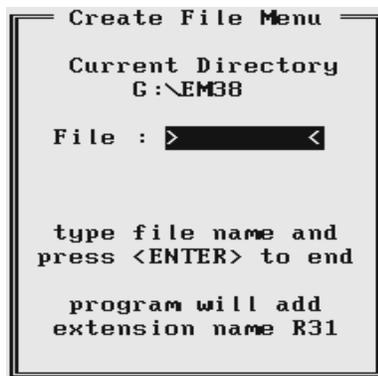
Each data file in the field computer (raw data file) has an extension name R31 and it is created in the programs current directory. The R31 files are created in the instrument binary format. They can be viewed using the Main menu option “View Files”. These files can be also converted to ASCII format and processed in the Geonics program DAT31W and DAT31 (for DOS).
