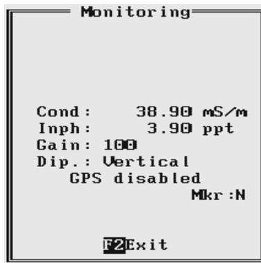
The EM31 readings are updated approximately 10 times per second during monitoring session. Values of conductivity in mS/m and Inphase in ppt are displayed. The dipole mode, instrument scale, and state of fiducial marker are continuously updated.
