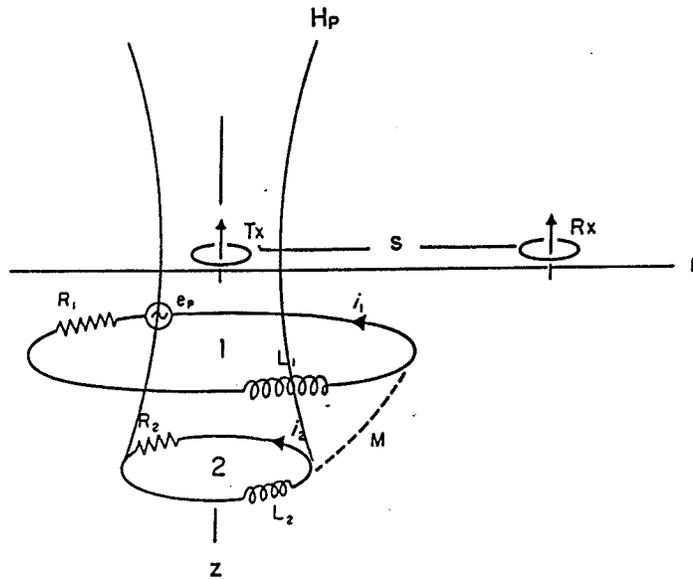
Figure 1. Electrical Model for Vertical Dipoles.
