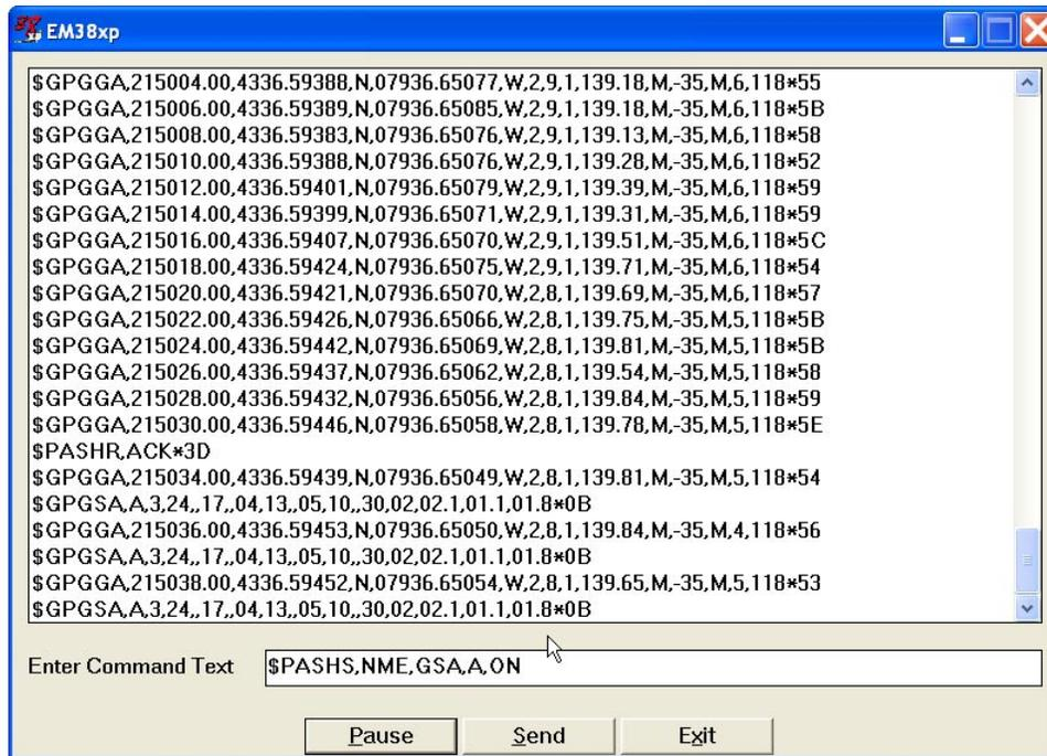
Please note, that not every GPS system accepts and uses the same standard set of NMEA commands and messages. In addition, some GPS systems do not accept commands sent by the serial port at all. The configuration of these type of receivers can be updated only by the controlling device (usually GPS logger, controller, or the receiver panel keys).
