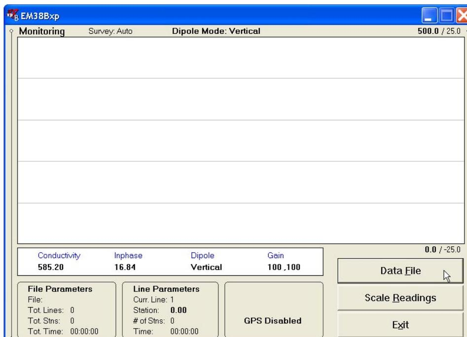
The remaining bottom section contains a window with current EM38B readings (Conductivity and Inphase, dipole mode, and Gain), three frames (File Parameters, Line Parameters, and GPS information), and command buttons located on the right side of the screen.
