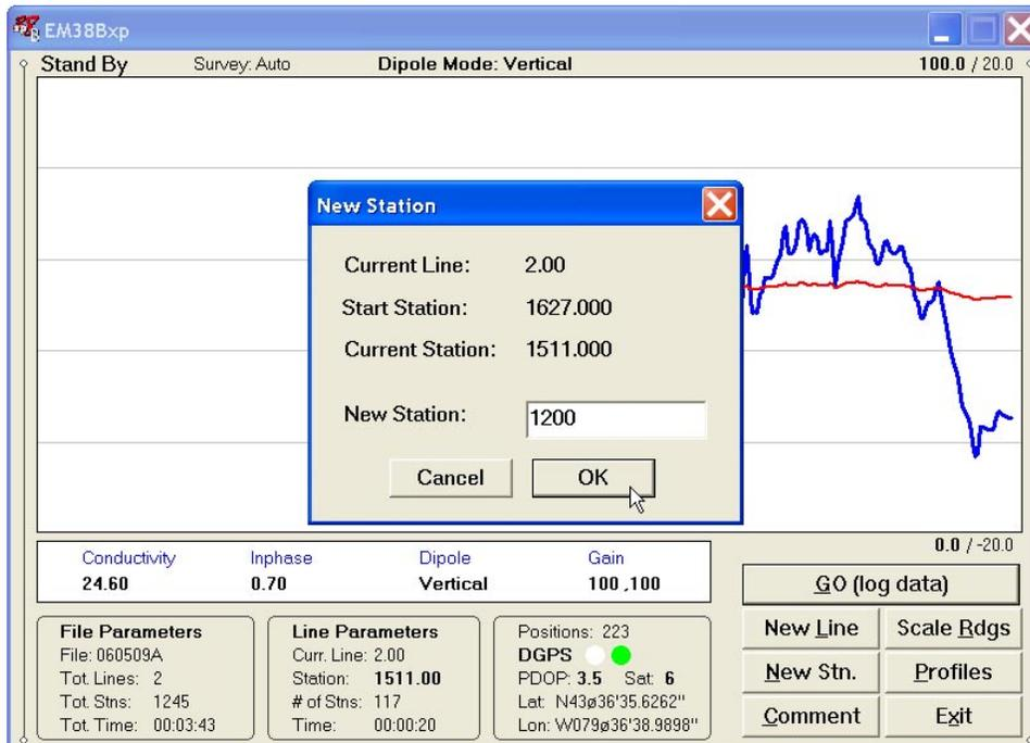
Current survey line, Start and Current station are displayed at the top of the dialog. The New Station can be entered in the provided edit box labeled New Station.
