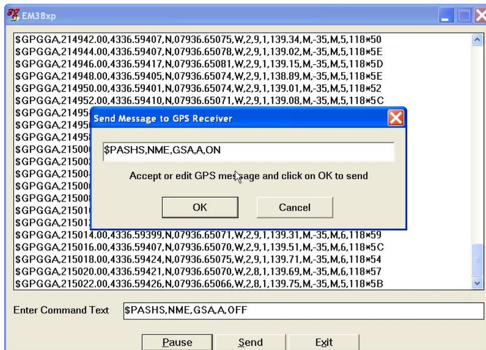
After this command is received by the GPS receiver, the confirmation message will be sent by the receiver (\$PASHR, ACK\*3D) and data stream will contain the message GSA (\$PASHR, NME,GSA,A,ON), see Figure below.
