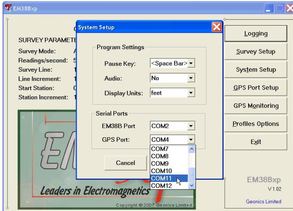
After all the parameters in the System Setup dialog are updated click on the button **OK** or press **ENTER** key to accept the displayed settings. The program will return to the Main Screen. Updated settings will be written to the initial file and they will be given as default parameters in the subsequent System Setup dialog.
