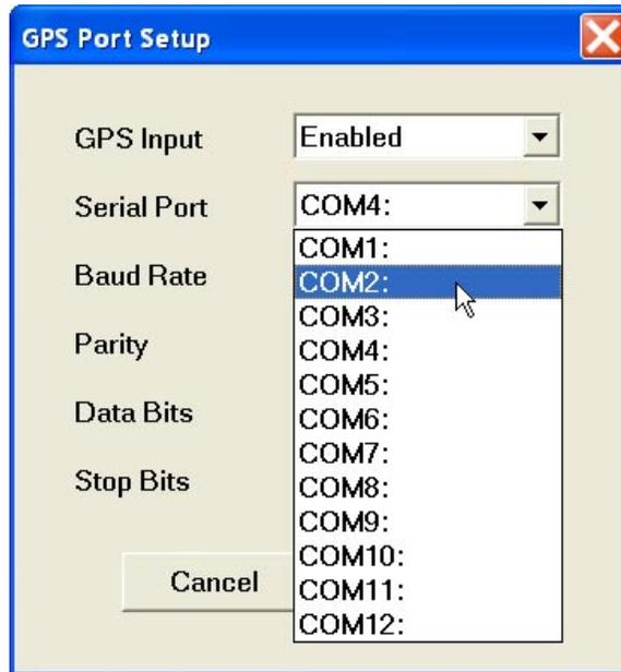
This port must be different than the port specified in the System Setup menu (for EM38B), otherwise a message will be displayed and ports will have to be reassigned.
