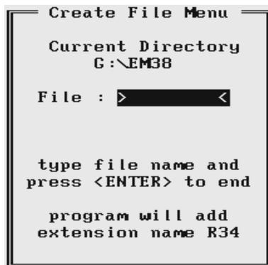
Each data file in the field computer (raw data file) has an extension name R34 and it is created in the programs current directory. The R34 files are created in the instrument binary format. They can be viewed using the Main menu option “View Files”. These files can be also converted to ASCII format and processed in the Geonics program DAT34W and DAT34RT (for DOS).
