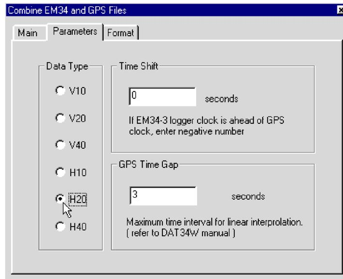
**Figure 8.6: Parameters page in the Combine EM34-3 and GPS Files window**
