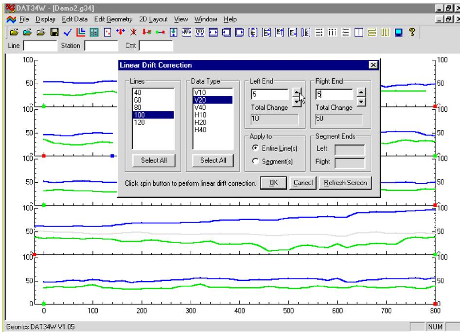
Figure 5.10: The DAT34W screen during Linear Drift Correction for the Entire Line
