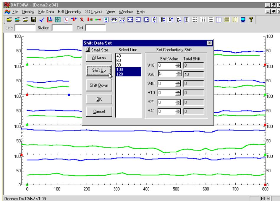
Figure 5.8: DAT34W screen during Shift Data procedure
