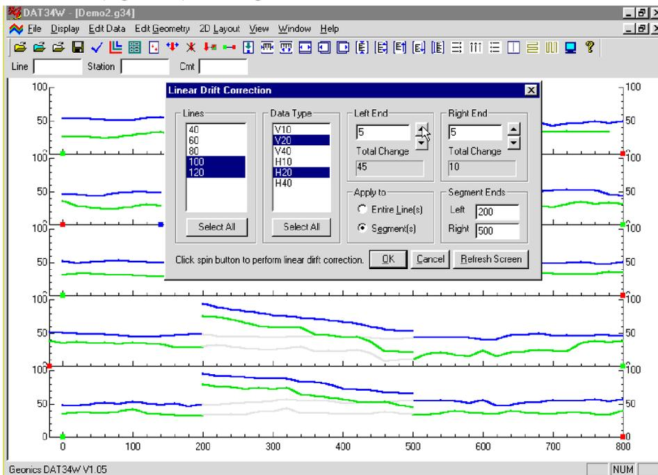
Figure 5.11: The DAT34W screen during Linear Drift Correction of Line Segments
