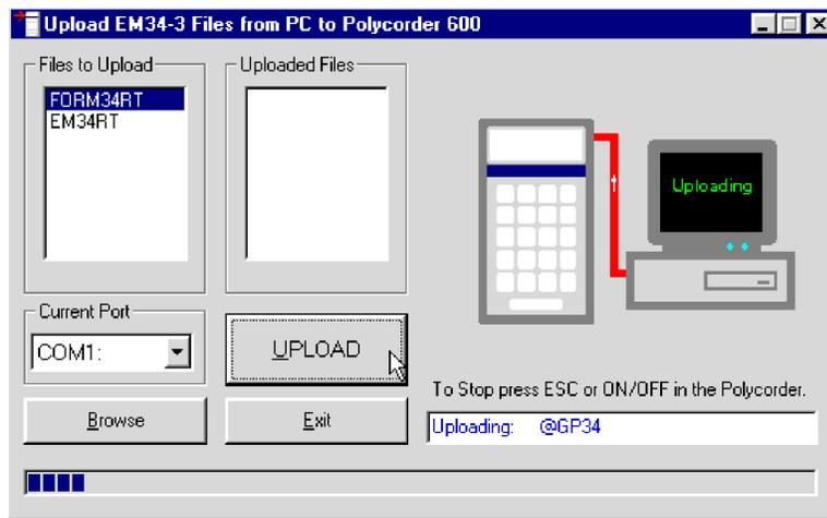
**Figure 3.5: Upload EM34 Files from PC to Polycorder 600 window during transmission**
