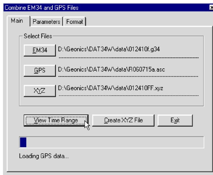
*Figure 8.8: Combine EM34-3 and GPS Files window during reading of EM34-3 and GPS files*
