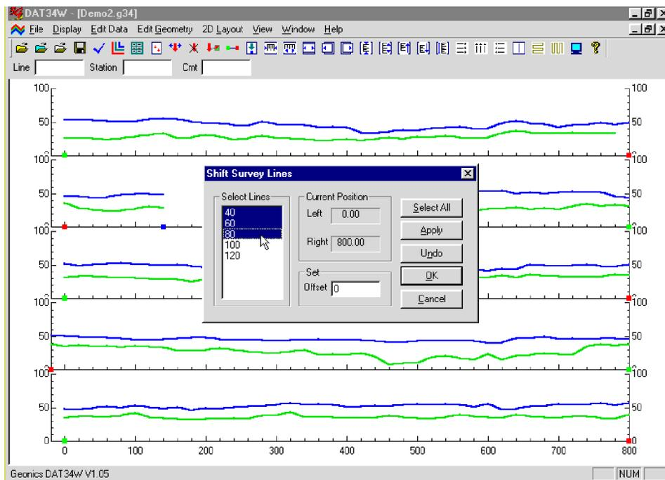
Figure 6.4: DAT34W screen with Shift Survey Lines window
