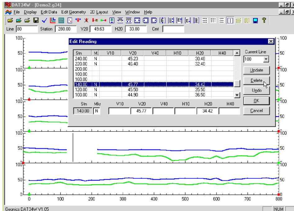
Figure 5.5: Edit Reading window during Delete Reading procedure
