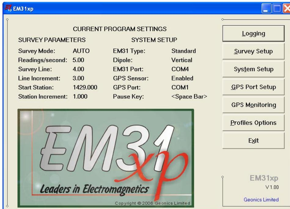
The Main Screen appears always as the first window after the program is started. It contains the name of the program, its version number (right bottom corner), and list of command buttons with available options on the right side. The major, left portion of the window contains information about current survey and system settings. This section is updated in real time as soon as the program parameters are changed in dialogs.
