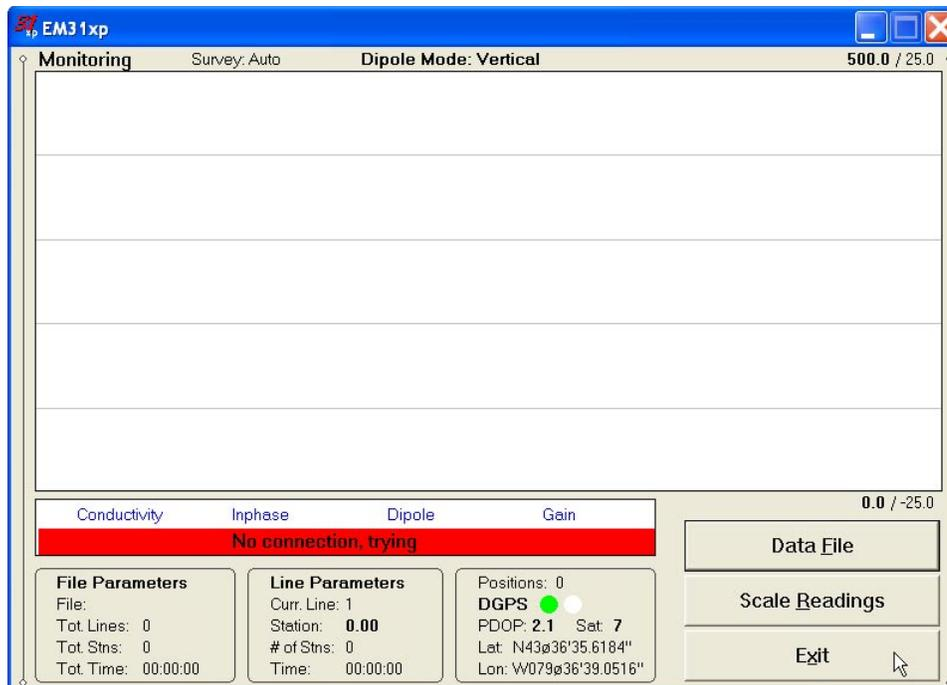
tor, Stand By or Logging), survey mode (Auto, Wheel, or Manual), and user specified instrument dipole mode (Vertical, Horizontal or Both following label **Dipole Mode:**). When fiducial marker is pressed then **M** is displayed.
