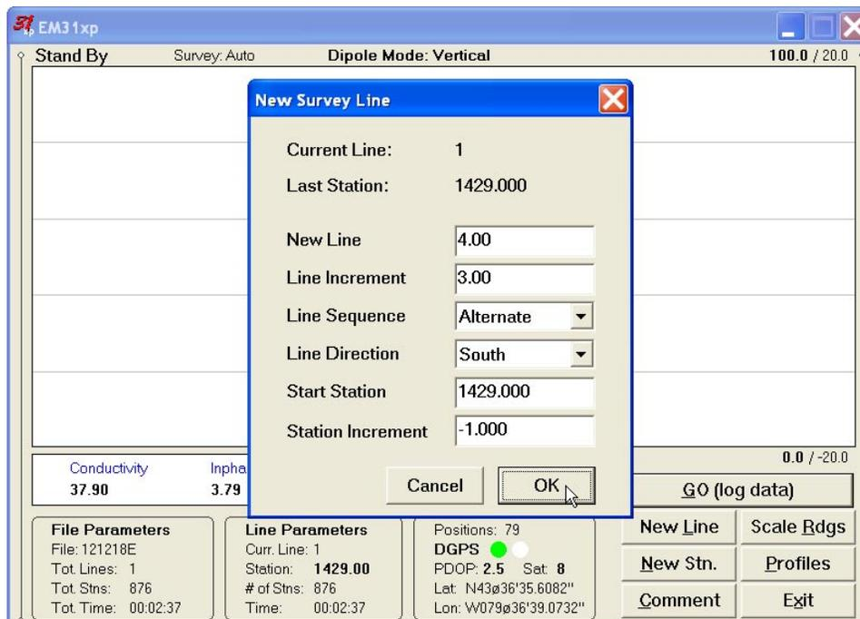
At the top of the dialog the last survey line name and the last logged station are displayed. Default name for the new line is given based on the Line Increment parameter. The default Start Station, direction of the Station Increment, and Direction are determined based on Sequence selection. All these parameters can be overwritten by the user as described in the Survey Setup menu description (chapter 2).
