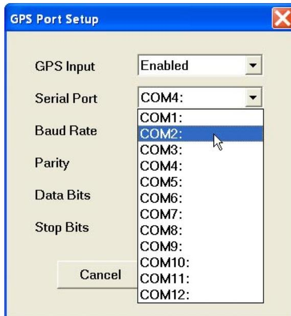
This port must be different than the port specified in the System Setup menu (for EM31), otherwise a message will be displayed and ports will have to be reassigned.
