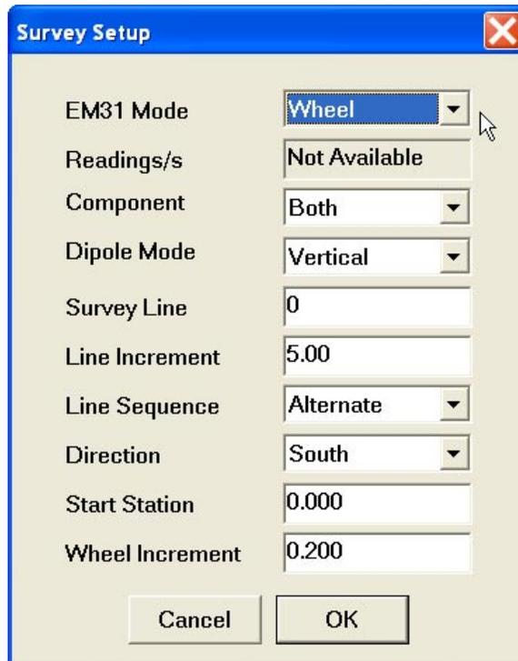
Please note that while in former data acquisition system (DAS70) Stn Increment (station increment) had only two options: Positive or Negative, in the current program this parameter is optional and its value has to be entered according to used wheel increment.
