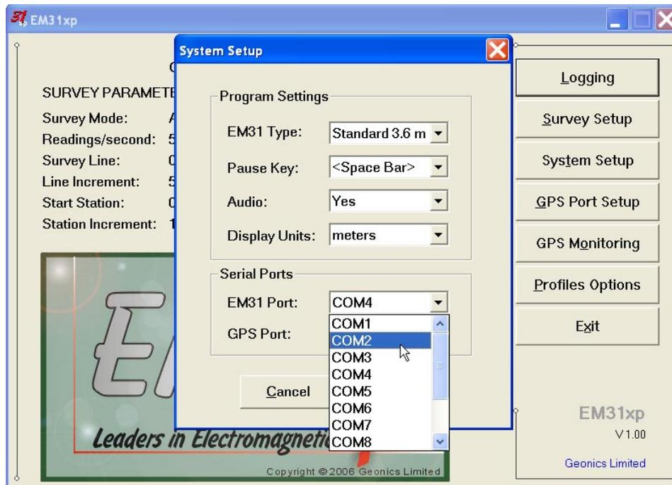
Select port number in the drop-down list box similarly to EM61-MK2 port assignment procedure.
