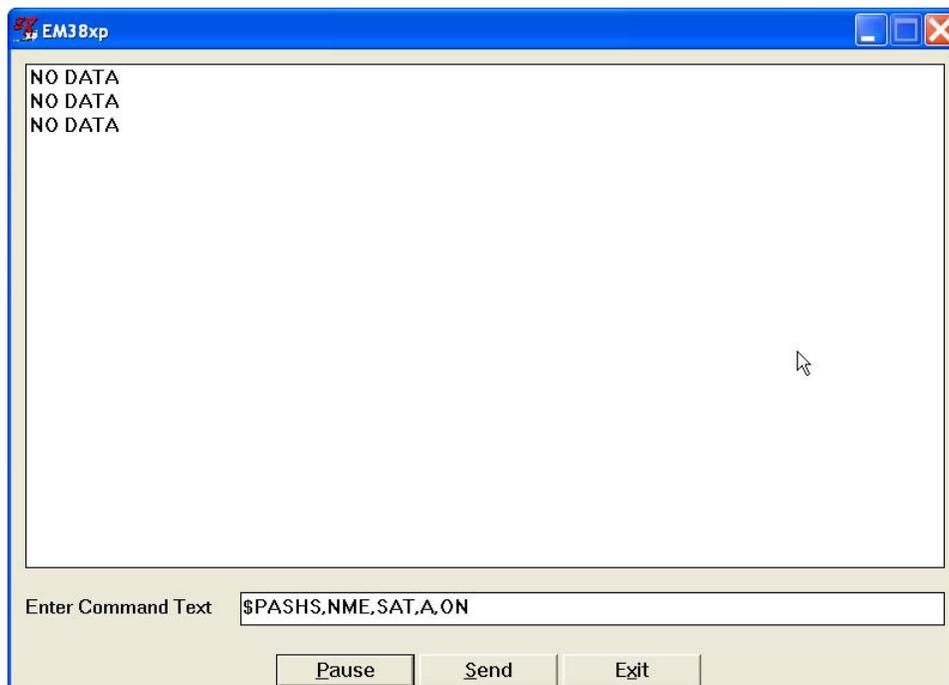
The message NO DATA is normally updated with a rate of 7 seconds. This may indicate the following: serial port number not correctly specified in Set Port for GPS dialog, GPS receiver not sending any data, and not working or not connected GPS receiver. If the message is updated more often than 7
