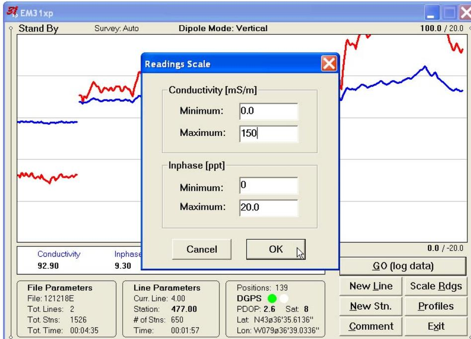
tings (minimum and maximum values) for the scale are displayed in the bottom right and top right corners of the plot area (Conductivity/Inphase). Values displayed in bold indicate the scale that is associated with grey grid lines.
