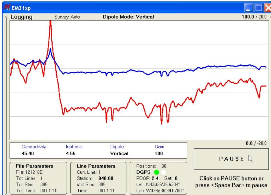
After the screen changes to Logging mode the current station (label **Stn:**) is updated according to the station interval. Similarly, if GPS Input was enabled, total number of GPS positions (label **Positions**) in the data file is incremented every time (usually once a second) GPS position is written
