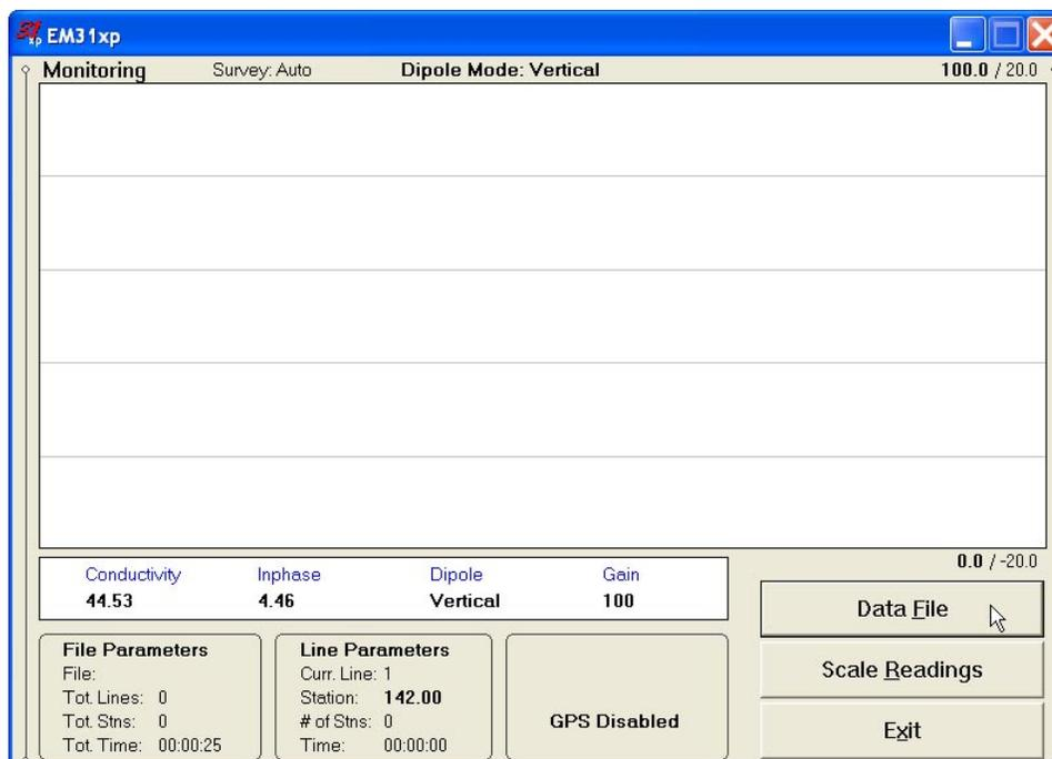
The remaining bottom section contains a window with current EM31 readings (Conductivity or Inphase, dipole mode, and Gain), three frames (File Parameters, Line Parameters, and GPS information), and command buttons located on the right side of the screen.
