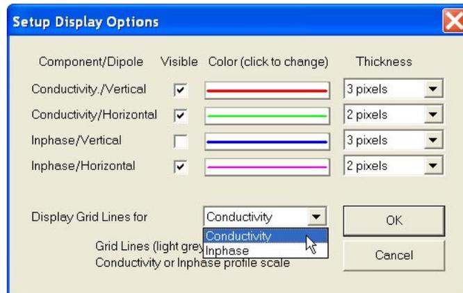
Minimum and maximum values for the component with selected grid lines are displayed as bold numerals. See figure below where grid lines are plotted for conductivity scale.
