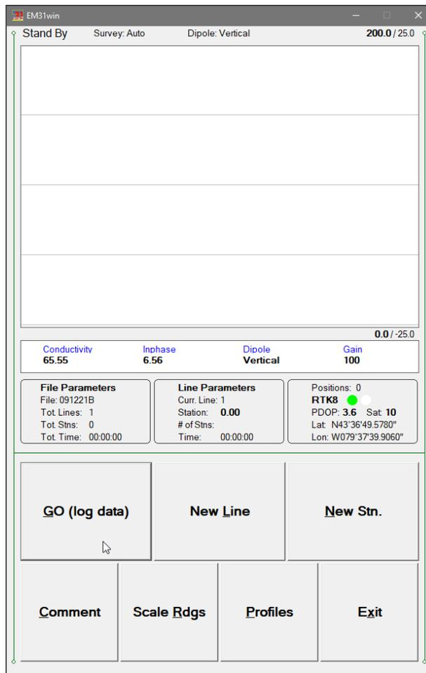
The main portion of the screen is occupied by the plot area which displays profiles (see Figure below which shows Stand By mode after some data were collected). Scale for conductivity and Inphase is labeled at the top and bottom of the plot window. The amplitude scale is divided by three to five
