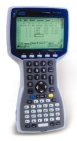
Additionally, and importantly, the Allegro includes two RS-232 serial input connections (and a user-accessible PC card slot) that facilitate the simultaneous collection of both EM and GPS data into a single data file. An optional Trimble Ag114 GPS, providing sub-metre accuracy, is available to support the requirement for position data.
