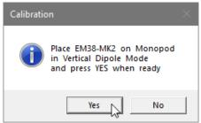
After the instrument is placed on the monopod in Vertical dipole mode click on the button **Yes** or press key **Y** (or **Enter** if button is highlighted). After button **Yes** was clicked a messages box disapears and a prompt **Vertical Calibration** is displayed (Figure below, on the left). From now on all messages and prompts will be written under plot section of the screen, in a line that is normally used to display labels for EM38-MK2 readings.
