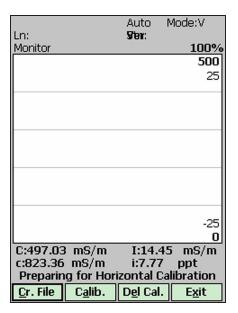
After a small delay required for stabilization the Horizontal Calibration will be performed.
