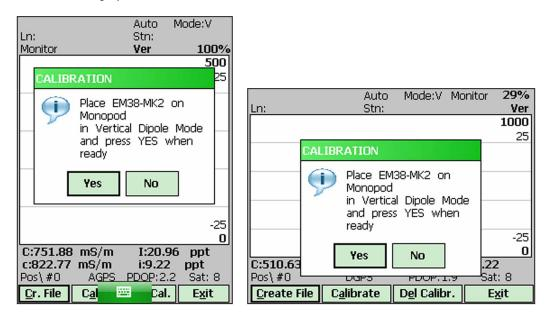
After the instrument is placed on the monopod in Vertical dipole mode tap button **Yes** or press key **Y** (or **Enter** if button is highlighted). After button **Yes** was tapped a messages box disapears and a prompt **Vertical Calibration** is displayed. From now on all mesages and prompts will be written under plot section of the screen, in a line that is normally used to display GPS parameters.
