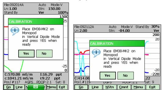
Calibration procedure is the same as described in chapter 6.1 (Monitoring Mode). Please refer to above section of the manual and follow all prompts that appear on the display. Calibration factors will be written to the data file and displayed readings will be adjusted immediately after the Calibration procedure is completed.
