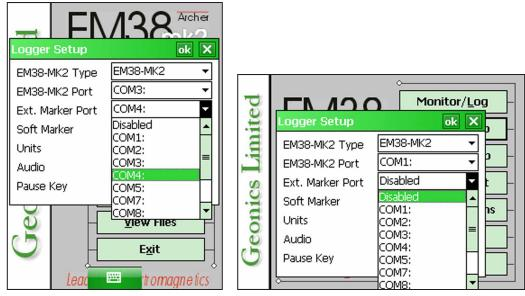
This port must be different than the port specified in the Set Port for GPS option (see next chapter), otherwise a message will be displayed and the ports will have to be reassigned. If External Marker is located on the Extender Arm then The EM38-MK2 and Ext. Marker Port must be the same (usually COM1 or COM2).
