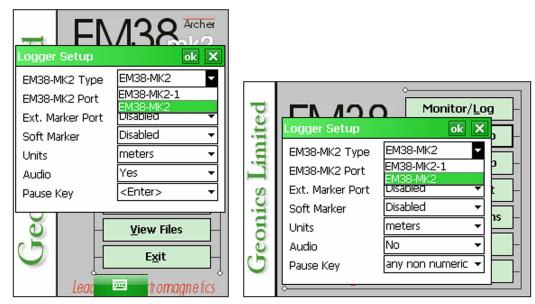
between the models is the number of included receiver coils: the EM38-MK2-1 includes one receiver coil with a 1 meter transmitter / receiver intercoil spacing; the EM38-MK2 includes two receiver coils with 0.5 and 1 meter intercoil spacings. The program default is the **EM38-MK2**.
