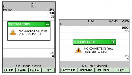
Check the connection or turn the instrument ON and select the Monitor/Log option again. Assuming that the instrument works properly the program will display the Monitor mode window. The layout of the Monitor window (for vertical and horizontal displayes) is as follows:
