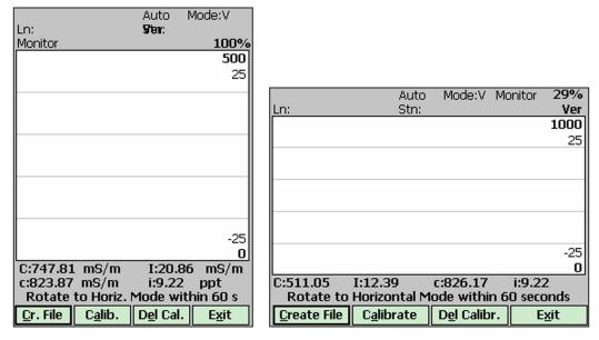
In cases where rotating the instrument takes longer than 1 minute the program will display the message "Horizontal Mode Failed - Wait for Beep", and after a short delay (about 2 seconds) the program will return to normal operation.
