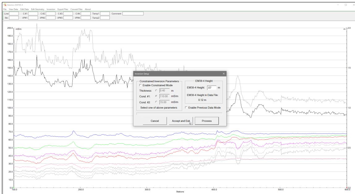
Figure 6.4 The DAT38-4 Inversion Setup dialog and display of profiles after calculations are completed.
