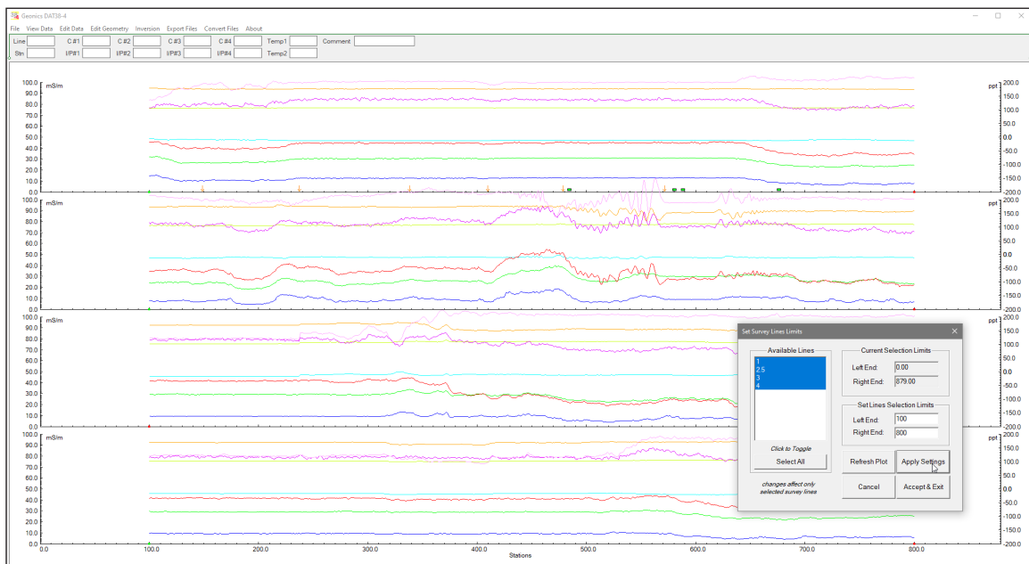
Figure 5.5 DAT38-4 profile display after action in Set Line Limits has been applied to all available survey lines.
