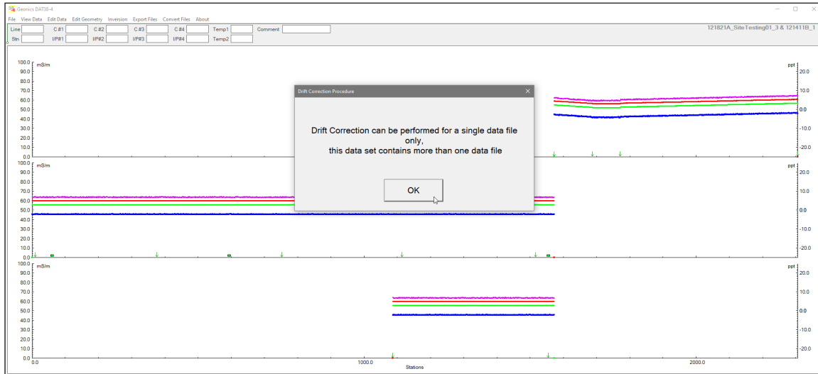
Figure 4.18 Warning message displayed when more than one data files are loaded and Drift Correction is attempted
