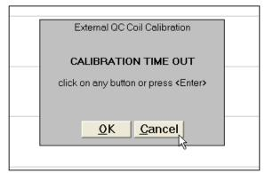
After pressing any key the program returns to Monitoring window. To repeat External QC coil calibration please tap the **Ext. QC.** button again.
