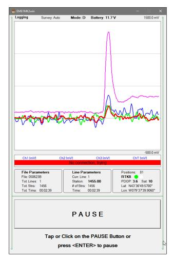
There is only one option available in the Logging mode - pause logging. After a Pause button is clicked or Pause key (any key or other Pause Key selected in Logger Setup window) is pressed the recording is stopped and the Logging mode returns to the Stand By mode. In Stand By mode the EM61-MK2 data will be displayed with the update rate approximately 10 readings per second, however data will not be saved in the log file and profile curves will be not updated.
