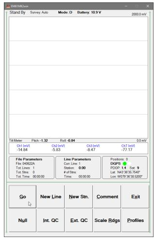
The main portion of the screen is occupied by the plot area which displays profiles (see Figure below which shows Stand By mode after some data were collected). Readings in the plot area can be displayed in compressed amplitude scale, which corresponds to Square Root of the amplitude. In compressed amplitude scale 0 to 100 corresponds to 0 to 10,000 mV, and compressed range 0 to 200 corresponds to 0 to 40,000 mV. Plotting data in compressed amplitude allows you to show
