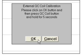
When External QC Coil Calibration window is displayed please use keyboard keys (O or C) rather than a mouse to execute buttons labeled OK and Cancel. Clicking on buttons by mouse will work, however several mouse button clicks may be required.
