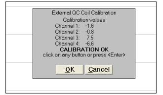
Otherwise, if the program determines that the reading is outside of the test values range the corresponding message "CALIBRATION FAILED" is displayed.
