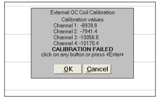
Regardless of the test result (OK or FAILED) the readings will be saved on screen. The program returns to Monitoring window after any button is clicked or ENTER key is pressed. Then the External QC coil calibration process can be repeated.
