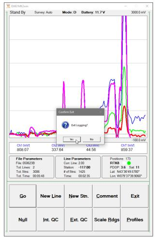
After above message is confirmed the program stops logging, closes data file and returns to Main Screen.
