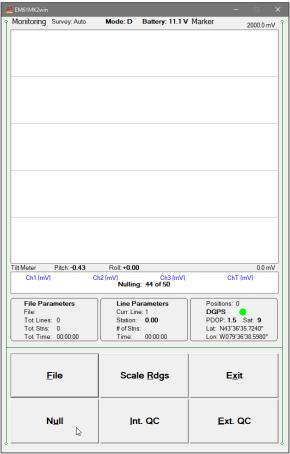
The calculated offset is applied to all the readings that follow this operation. If needed, this procedure can be repeated several times until satisfactory results are obtained. However, there is no associated "Undo" function. If original values (without calculated offsets) of the EM61-MK2 readings are needed, exit the EM61MK2 program and run it again. The EM61-MK2 instrument does not have to be turned OFF. Null operation can be also performed later during data collection.
