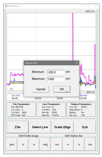
To shift the range of the displayed stations and to move the vertical bar indicating the currently displayed station, use the buttons located along the bottom of the View Files window. These buttons can be activated by tapping or by pressing the keyboard keys. They are divided in two groups: four buttons labeled Shift Profile Image are used to move image while four buttons labeled Shift Station Bar move grey vertical bar selecting current station and displaying its numeric values.
