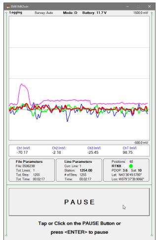
After the screen changes to Logging mode the current station (labeled **Station**:) is updated according to the station interval. Similarly, if GPS Input was enabled, total number of GPS positions (label **Positions**) in the data file is incremented every time (usually once a second) GPS position is written to the file. Profile curves (for channels selected in Display Options window) are updated after each reading is written to the data file.
