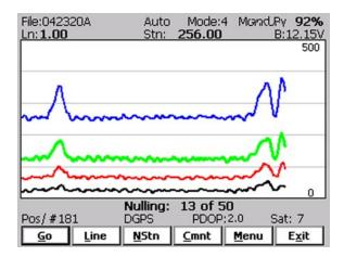
The calculated offset is applied to all the readings that follow this operation. If needed, this procedure can be repeated several times until satisfactory results are obtained. However, there is no associated "Undo" function. If original values (without calculated offsets) of the EM61-MK2 readings are needed, exit the EM61MK2 program and run it again. The EM61-MK2 instrument does not have to be turned OFF.
