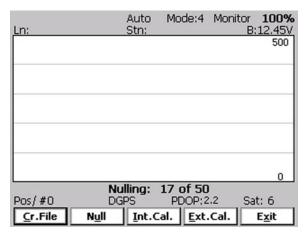
The calculated offset is applied to all the readings that follow this operation. If needed, this procedure can be repeated several times until satisfactory results are obtained. However, there is no associated "Undo" function. If original values (without calculated offsets) of the EM61-MK2 readings are needed, exit the EM61MK2 program and run it again. The EM61-MK2 instrument does not have to be turned OFF. Null operation can be also performed later during data collection.
