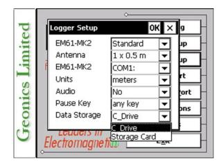
After all the parameters in the Logger Setup dialog are updated tap the button **OK** or press **ENTER** key to accept the displayed settings. The program will return to the Main Screen. Updated settings will be written to the initial file and they will be given as default parameters in the subsequent Logger Setup dialog.
