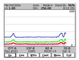
Readings for channels 1, 2, 3, and 4 (or T) are shown in numeric form below the plot area. Channel labels are not displayed due to the small screen of the Allegro. Values of readings are displayed in the following order (from the left): Channel 1, 2, 3, and 4 (or T). EM61-MK2 readings (in numeric form) are updated in Stand By mode approximately 10 times per second. Profiles in the plot area are updated only during Logging mode when data are actually saved in the data file.
