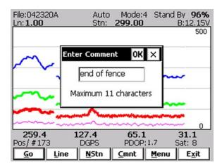
Tap the button **OK** or press **ENTER** key to accept the comment entered in a text box of the dialog. The text of the comment is saved in the file with a corresponding time stamp and the program will return to the Logging window in Stand By mode.
