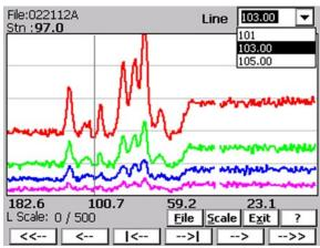
To shift the range of the displayed stations and to move the vertical bar indicating the currently displayed station, use the buttons located along the bottom of the View Files window. These buttons can be activated by tapping or by pressing the keyboard keys. A help screen containing info related to each button can be displayed at any time by tapping (or executing from keyboard) the Help button labeled ?. The Help screen is shown below.
