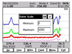
After minimum and maximum values are specified tap the button **OK** or press **ENTER** key to accept to accept new values and the profile plot area will be redrawn (see Figure below).
