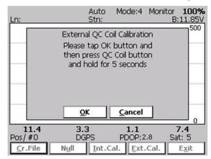
After **OK** button is tapped (or shortcut key **O** is pressed) the window displays timer with elapsed seconds and EM61-MK2 readings. This display lasts for 60 seconds. During this time please follow the instructions provided on the Allegro screen.
