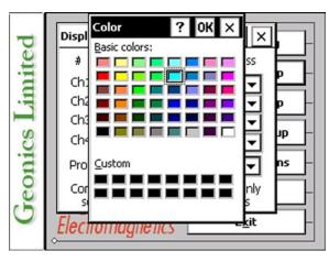
Select desired colour by tapping on a colour box (the selected colour box will be high-lighted).
