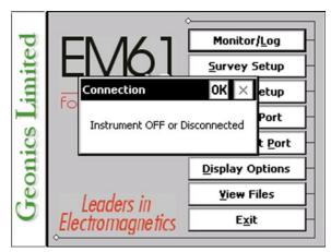
Check the connection or turn the instrument ON and select the Monitor/Log option again.
