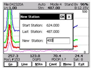
Start and Current station are displayed at the top of the dialog. The New Station can be entered in the provided edit box labeled New Station.
