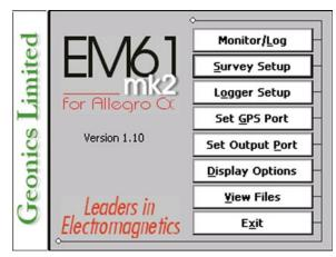
These options are selected by using tapping buttons, or from keyboard using TAB/ENTER or shortcuts indicated by underline label characters. In case of Main Screen buttons the **Down** and **Up** arrow keys and **<ENTER**> can be used as well.
