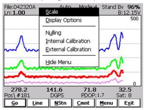
The Enter Scale dialog will be displayed. It contains two text boxes for Minimum and Maximum values of a new scale for profile plot. Current settings (minimum and maximum values) for the scale are displayed in the bottom right and top right corners of the plot area.
