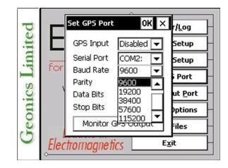
Tapping on the down arrow next to the text box labeled Baud Rate opens a drop-down box showing the available parameters, or when the keyboard is used activate this text box by pressing TAB key and then by using up or down arrow keys select one of available items.
