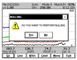
After above message is confirmed the program collects 50 readings and calculates the instrument offset.
