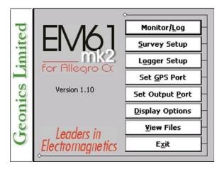
parameters can be quickly examined and some functions (creating data file, nuling, QC coil check) can be performed. After a data file is created in Monitoring mode, the program switches to Stand By mode and allows access to Logging mode. In Stand By mode instrument output can be monitored and some survey and logging parameters can be changed, and Logging mode is used only to record data. Two modes Stand By and Logging are toggled by **GO** and **Pause** buttons.
