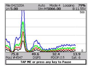
After the screen changes to Logging mode the current station (label **Stn:**) is updated according to the station interval. Similarly, if GPS Input was enabled, total number of GPS positions (label **Pos**) in the data file is incremented every time (usually once a second) GPS position is written to the file. Profile curves (for channels selected in Display Options window) are updated after each reading is written to the data file.
