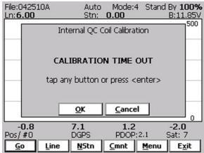
After pressing any key the program returns to logging window in Stand By mode. To repeat Internal QC coil calibration please repeat the procedure.
