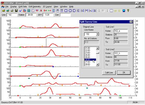
Figure 6.8: Profile View display before survey line split
