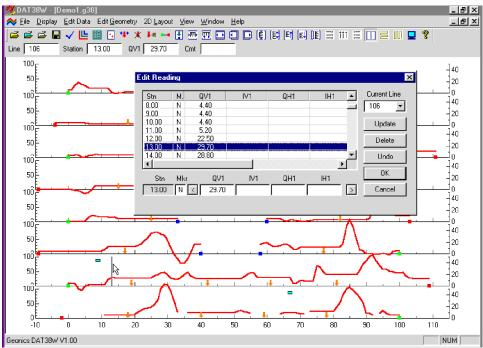
Figure 5.4: Edit Reading window with a vertical bar indicating position of the station in the profile view.
