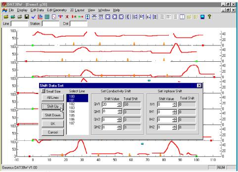
Figure 5.8: DAT38W screen during Shift Data procedure
