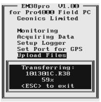
Figure 3.20: Pro4000 screen during data transfer
