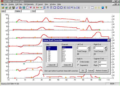
Figure 5.11: The DAT38W screen during Linear Drift Correction of Line Segments
