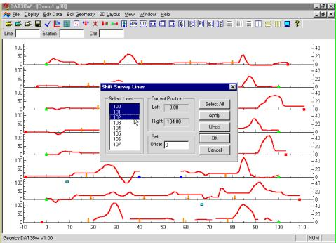
Figure 6.4: DAT38W screen with Shift Survey Lines window
