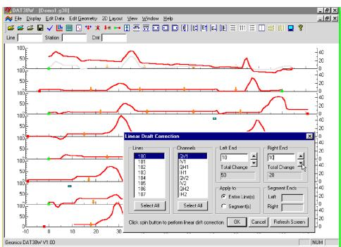
Figure 5.10: The DAT38W screen during Linear Drift Correction for the Entire Line
