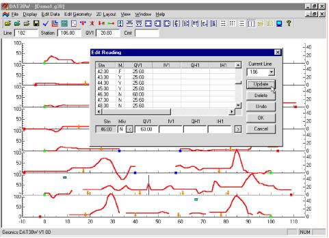
Figure 5.6: Edit Readings window during editing value of readings
