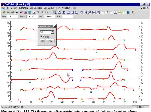
Figure 6.18: DAT38W screen after positioning group of selected end stations (compare Figure 6.17)
