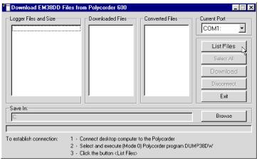
Figure 3.7: Download EM38 DDFiles from Polycorder window
