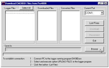
Figure 3.13: Download EM38DD Files from Pro4000 window
