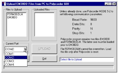
Figure 3.3: Selecting serial port number
