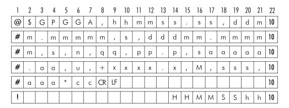
The GPS sequence may contain 5 or 6 records. Component of the GGA message may differ in length, however they are placed in the same number of columns. Refer to EM38Dpro Users Manual Appendix A (section A.2) for definition of each component of GGA data message.
