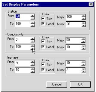
Figure 4.17: Set Display Parameters window
