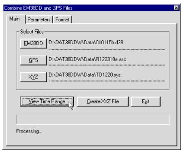
Figure 8.8: Combine EM38DD and GPS Files window during reading of EM38DD and GPS files
