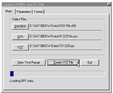
Figure 8.10: Combine EM38 and GPS Files window during reading data files and creating output XYZ file
