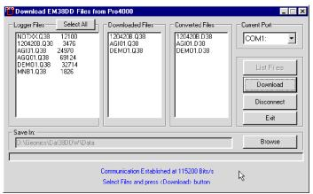
Figure 3.21: Download EM38DD Files from Pro4000 after downloading selected files is completed
