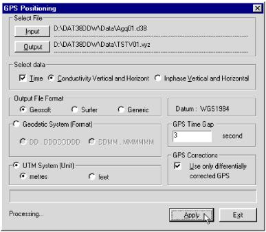
Figure 8.16: GPS Positioning window during creating XYZ (output) file
