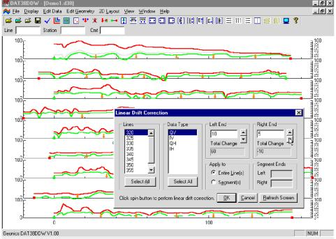
Figure 5.10: The DAT38DDW during Linear Drift Correction for the Entire Line
