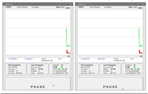
right show the second reading taken. The program keeps track of number of readings (number of Configurations) at each station. It is up to operator to set instrument to desired Dipole Mode and Coil Separation for each reading.
