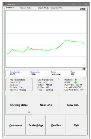
label. Readings are followed by current coil separation (10, 20, or 40 m), dipole mode (Vertical or Horizontal) and EM34-3 currently set range (labeled **Gain**). EM34-3 readings (in numeric form) are updated in Stand By mode approximately 10 times per second. Profiles in the plot area are updated only during Logging mode when data are actually saved in the data file.
