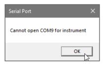
Check the connection, change settings, or turn the instrument ON and select the Logging option again.
