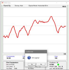
After above message is confirmed the program stops logging, closes data file and returns to Main Screen.
