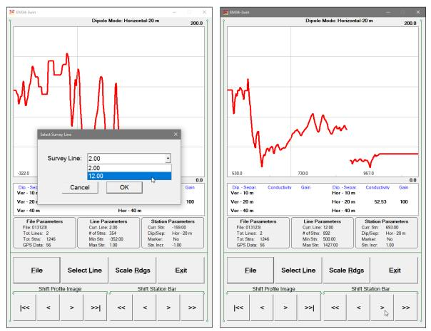
To change the currently displayed survey line click or tap on the button labeled Select Line. A dialog labeled Select Survey Line will be displayed (Figure below on the left).
