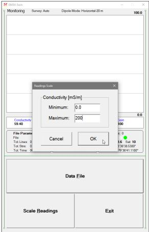
After minimum and maximum values are specified tap the button **OK** or press **ENTER** key to accept new values and the profile plot area will be redrawn.
