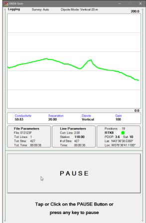
There is only one option available in the Logging mode - pause logging. After a Pause button is clicked or Pause key (any key or other Pause Key selected in Logger Setup window) is pressed the recording is stopped and the Logging mode returns to the Stand By mode. In Stand By mode the EM34-3 data will be displayed with the update rate approximately 10 readings per second, however data will not be saved in the log file and profile curves will be not updated.
