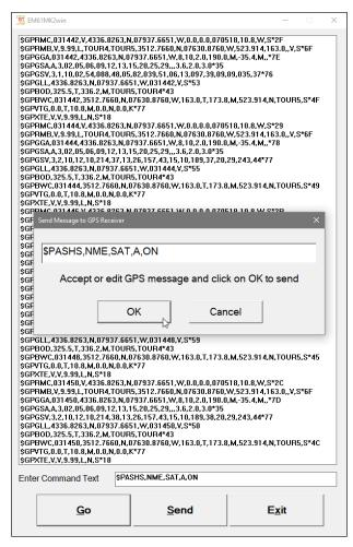
After this command is received by the GPS receiver, the confirmation message will be send by the receiver (\$PASHR, ACK\*3D) and data stream will contain the message SAT if it is available in the connected GPS receiver.
