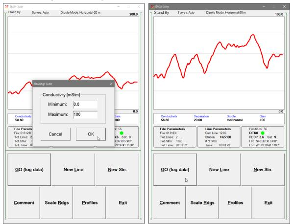
After minimum and maximum values are specified click on the button **OK** or press **EN-TER** key to accept new values and the profile plot area will be redrawn (see Figure above on the right).
