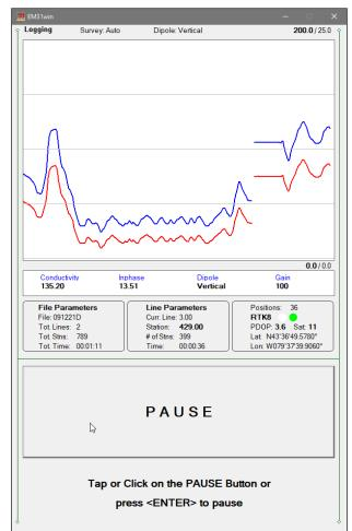
After the screen changes to Logging mode the current station (labeled **Station:**) is updated according to the station interval. Similarly, if GPS Input was enabled, total number of GPS positions (label **Positions**) in the data file is incremented every time (usually once a second) GPS position is written to the file. Profile curves (for channels selected in Display Options window) are updated after each reading is written to the data file.
