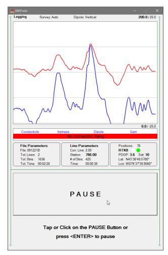
There is only one option available in the Logging mode - pause logging. After a Pause button is clicked or Pause key (any key or other Pause Key selected in Logger Setup window) is pressed the recording is stopped and the Logging mode returns to the Stand By mode. In Stand By mode the EM31-MK2 data will be displayed with the update rate approximately 10 readings per second, however data will not be saved in the log file and profile curves will be not updated.
