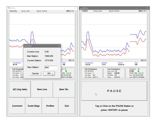
Current survey line, Start and Current station are displayed at the top of the dialog. The New Station can be entered in the provided edit box labeled New Station.
