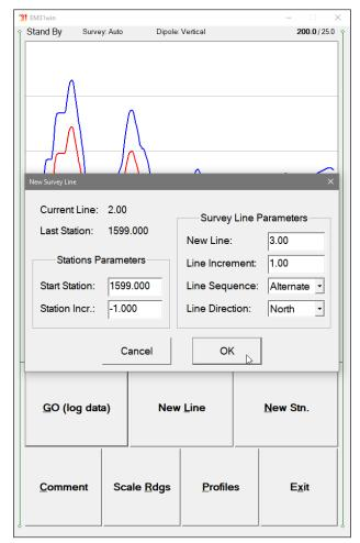
At the top of the dialog the last survey line name and the last logged station are displayed. Default name for the new line is given based on the Line Increment parameter. The default Start Station, direction of the Station Increment, and Direction are determined based on Sequence selection. All these parameters can be overwritten by the user as described in the Survey Setup menu description (chapter 2).
