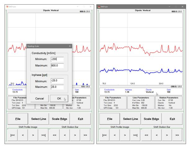
To shift the range of the displayed stations and to move the vertical bar indicating the currently displayed station, use the buttons located along the bottom of the View Files window. These buttons can be activated by tapping or by pressing the keyboard keys. They are divided in two groups: four buttons labeled Shift Profile Image are used to move image while four buttons labeled Shift Station Bar move grey vertical bar selecting current station and displaying its numeric values.
