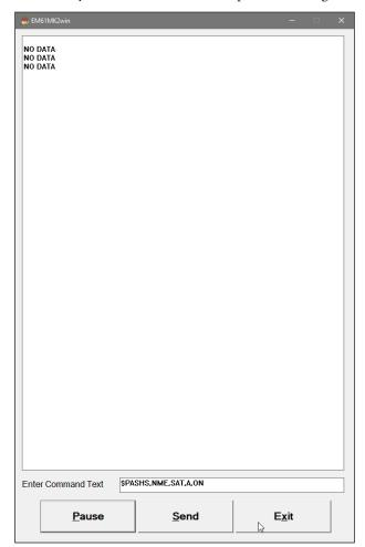
The monitoring display can be stopped any time by using button labeled **Pause**. At that time scrolling of the GPS output will be stopped, and the button will be labeled **Go**. The next click (or keyboard action) on this button will activate receiving and display of GPS data.
